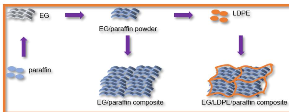
**Figure 2.** Preparation diagram of EG/paraffin composite and EG/LDPE/paraffin composite.
