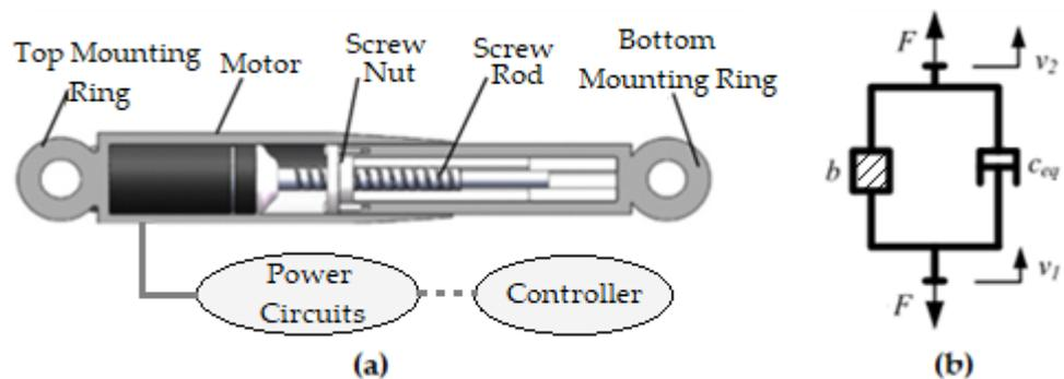
**Figure 13.** Structural diagram of the ball screw of the shock absorber—(a) and equivalent to the dynamic model—(b).
