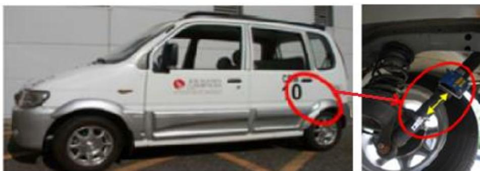
**Figure 14.** Location of the shock absorber to collect energy in the minivan vehicle [219].
