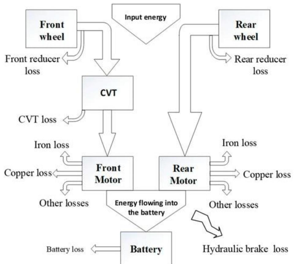
Figure 9. Graph of energy consumption and losses during braking [194].
