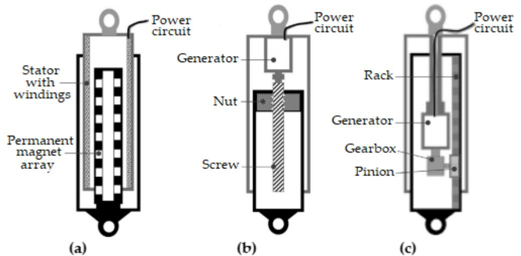
**Figure 12.** The electromagnetic regenerative shock absorbers (a) linear motor, (b) ball screw and (c) rack-pinion.
