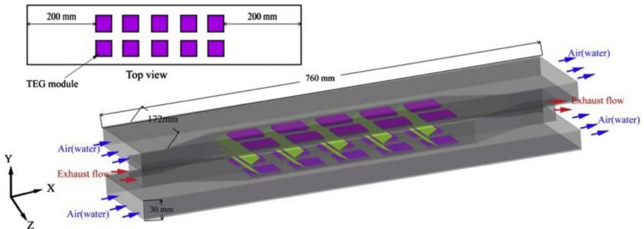
**Figure 5.** An example of a thermoelectric generator system for energy recovery from ICE exhaust [140].
