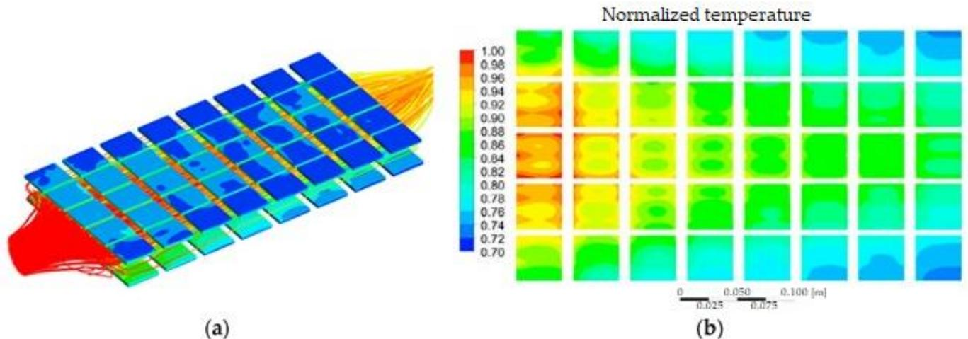
**Figure 7.** (a) Simulation of flue gas flow in the TEG module and (b) temperature distribution in the modules (upper surfaces) [184].
