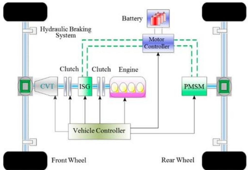
Figure 8. Schematic diagram of dual motor hybrid electric vehicle [194]. CVT—continuously variable transmission; PMSM—permanent magnet synchronous motor; ISG—integrated starter generator.
