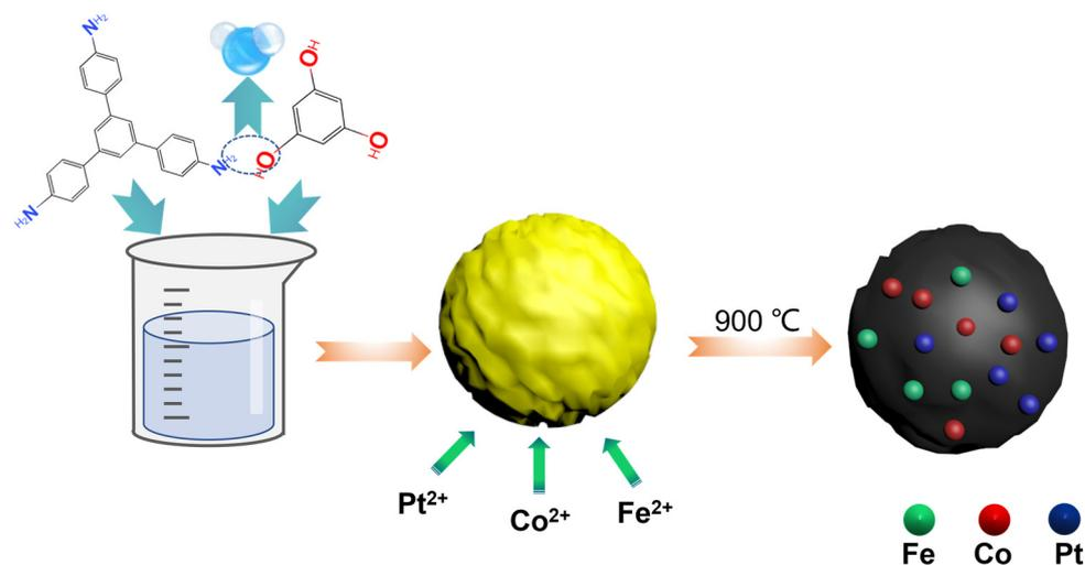
**Figure 1.** Synthesis process of Pt, Fe, Co/N-C.
