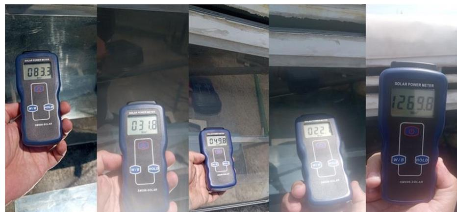
**Figure 17.** Reflected surface radiation of TTI filled with R1233zd.
