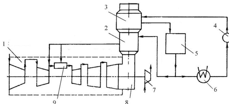
**Figure 1.** The scheme of the “Aquarius” type power plant: 1—gas turbine engine; 2—waste heat boiler; 3—steam-gas condenser; 4—electric pump; 5—condensate collector; 6—cooler; 7—power consumer; 8—gas outlet; 9—gas turbine combustion chamber.
