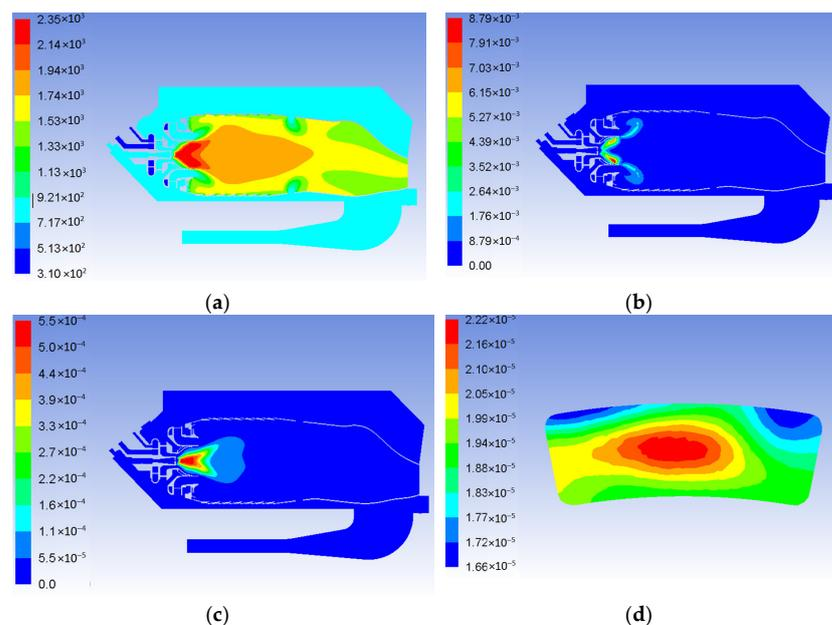
**Figure 12.** Contours of temperature (a), mass fraction of CO (b), mass fraction of NO (c) in longitudinal section, and mass fraction of NO at the outlet (d) for the premixed combustion chamber at 20%  $H_2$  (by volume).
