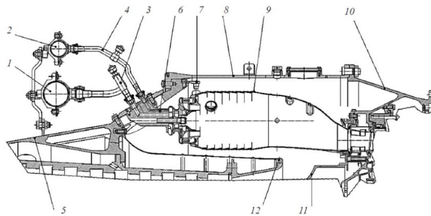
**Figure 2.** Combustion chamber with pre-mixing of components: 1, 2—fuel collectors; 3, 4—fuel supply lines; 5—casing of compressor; 6—burner; 7—spacer; 8—frame; 9—flame tube; 10—turbine casing; 11—diffuser; 12—housing.
