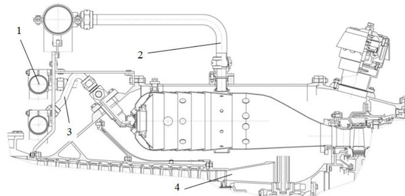
**Figure 3.** Combustion chamber of the “Aquarius” gas–steam power plant with steam injection: 1—ecological steam supply; 2—energy steam supply; 3—fuel supply; 4—air inlet.
