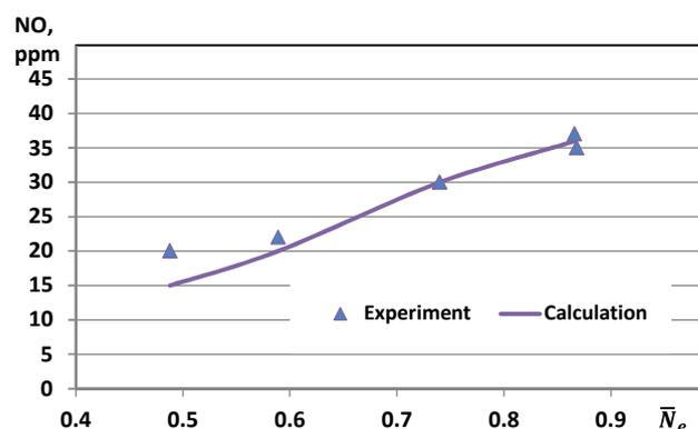
**Figure 5.** Computed and experimental concentrations of nitrogen oxides in the combustion chamber with steam injection.
