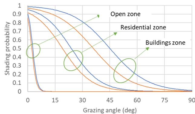
**Figure 11.** Shading distribution on three zones used for the resilience probability; blue curves correspond to the x-direction (left–right direction), and the red curves correspond to the y-direction (front–rear).
