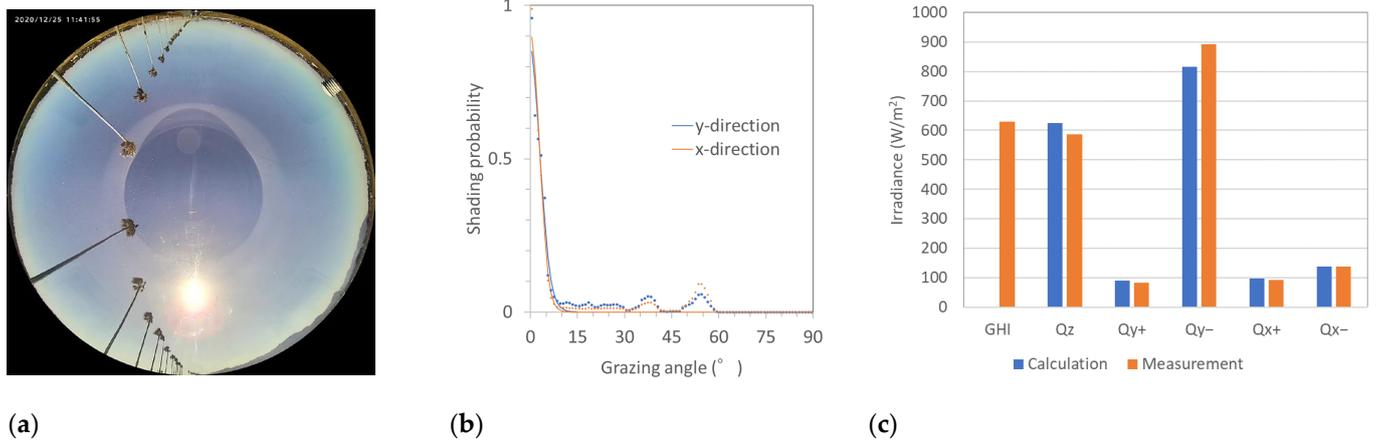
**Figure 8.** Shading distribution and irradiance onto VIPVs (5-axis) of the open zone: (a) fisheye image; (b) shading probability as the function of the grazing angle; (c) comparison of the measured (red bars) and calculated (blue bars) irradiance onto 5-axis planes.
