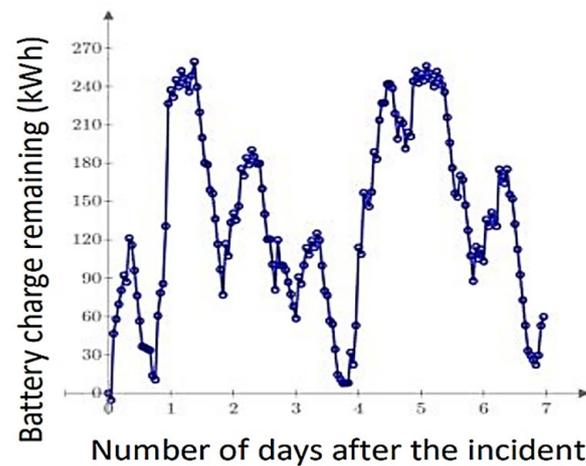
**Figure 13.** Monte Carlo simulation result: A time-series plot of the total battery charge remaining in the facilities supported by SEVs.
