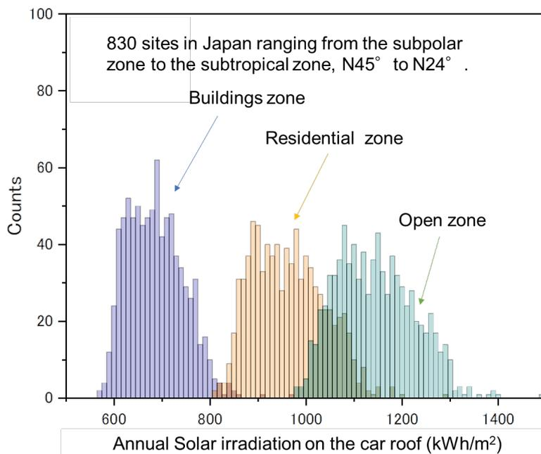
**Figure 19.** Histogram of the estimated solar irradiance on a car roof in Japan from 830 sites (N45° to N24°, ranging from subpolar to subtropical zone) in three zones.
