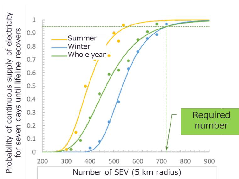
**Figure 15.** Number of SEVs vs. probability of continuous electricity supply for seven days, until the lifeline recovers (residential zone in Miyazaki).
