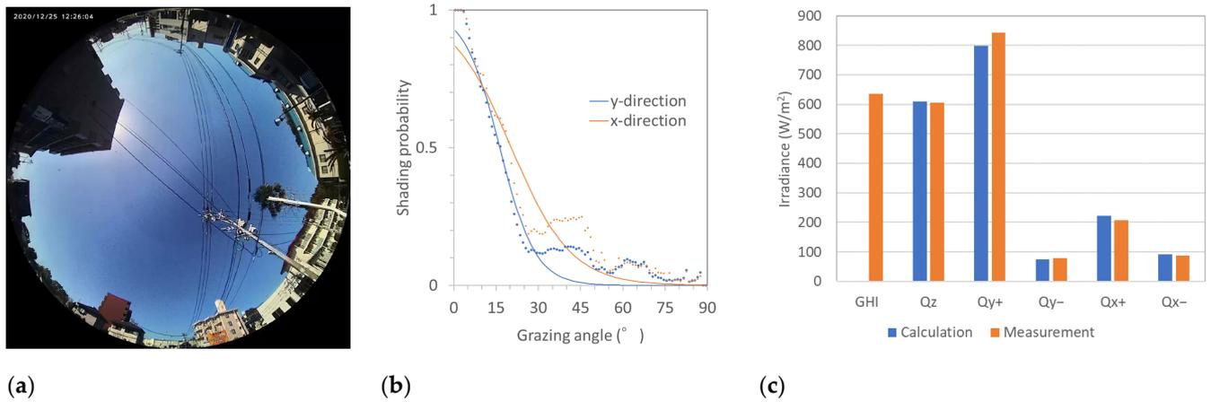
**Figure 9.** Shading distribution and irradiance onto VIPVs (5-axis) of the residential zone: (a) fisheye image; (b) shading probability as the function of the grazing angle; (c) comparison of the measured (red bars) and calculated (blue bars) irradiance onto 5-axis planes.
