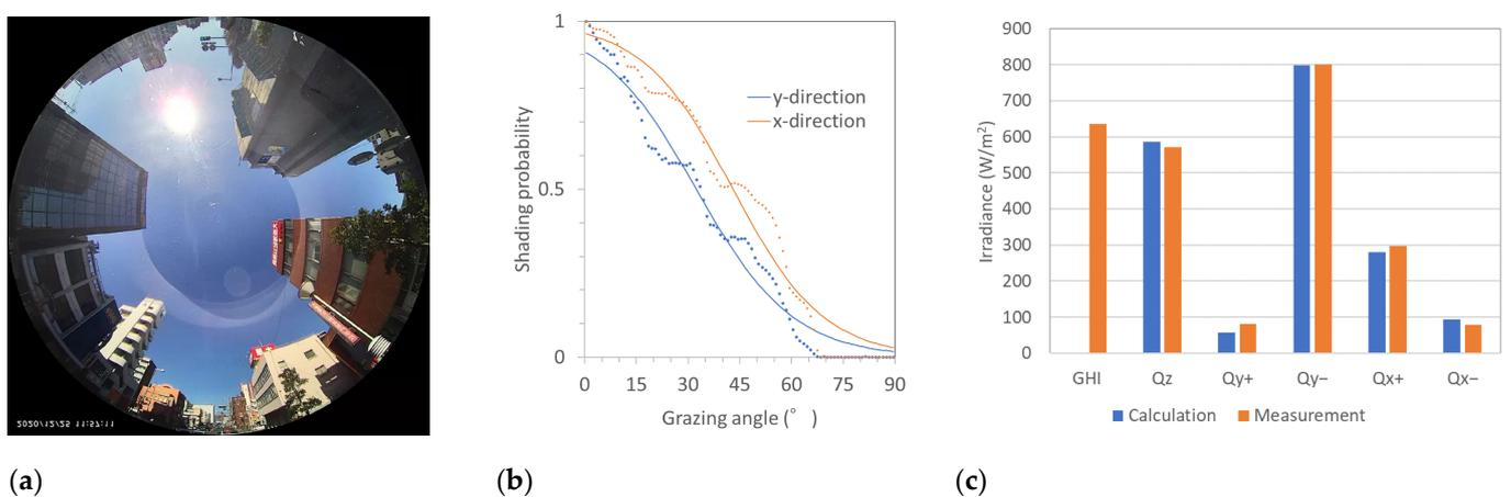
**Figure 10.** Shading distribution and irradiance onto VIPVs (5-axis) of the building zone: (a) fisheye image; (b) shading probability as the function of the grazing angle; (c) comparison of the measured (red bars) and calculated (blue bars) irradiance onto 5-axis planes.
