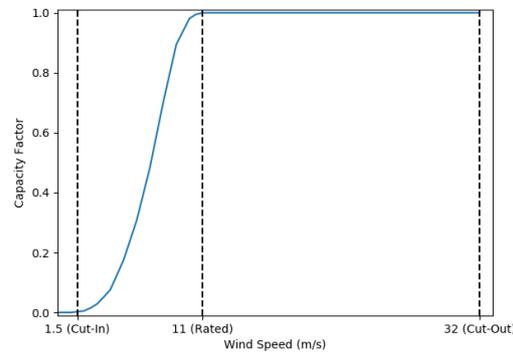
**Figure 2.** Wind turbine power curve used, with bounding curve calculated from all available turbine data provided by the Open Energy Platform [31].
