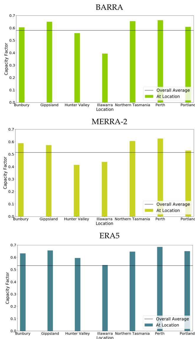
**Figure 5.** Average capacity factor (2009–2018) predicted using each dataset for key locations compared to whole-domain average
