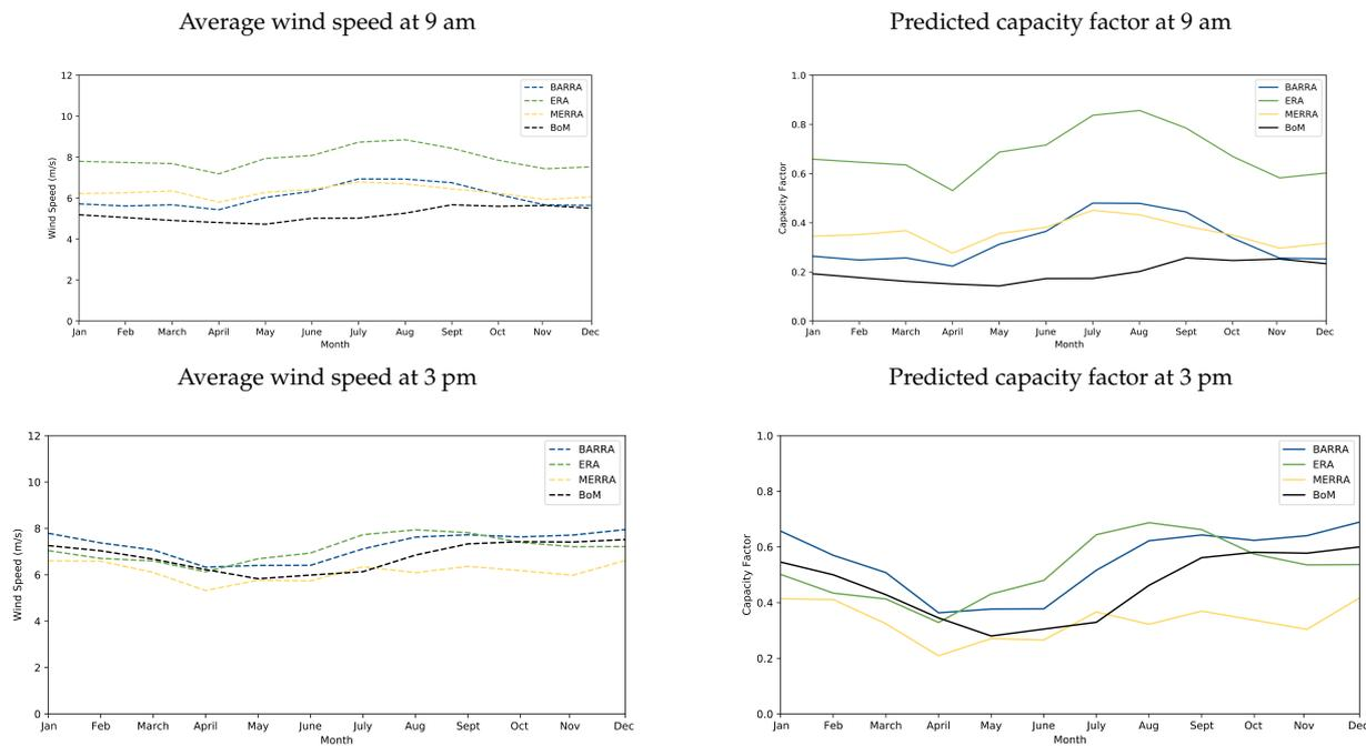
**Figure 12.** Comparison between average wind speed at 150 m across key locations and corresponding capacity factor predicted using each data source
