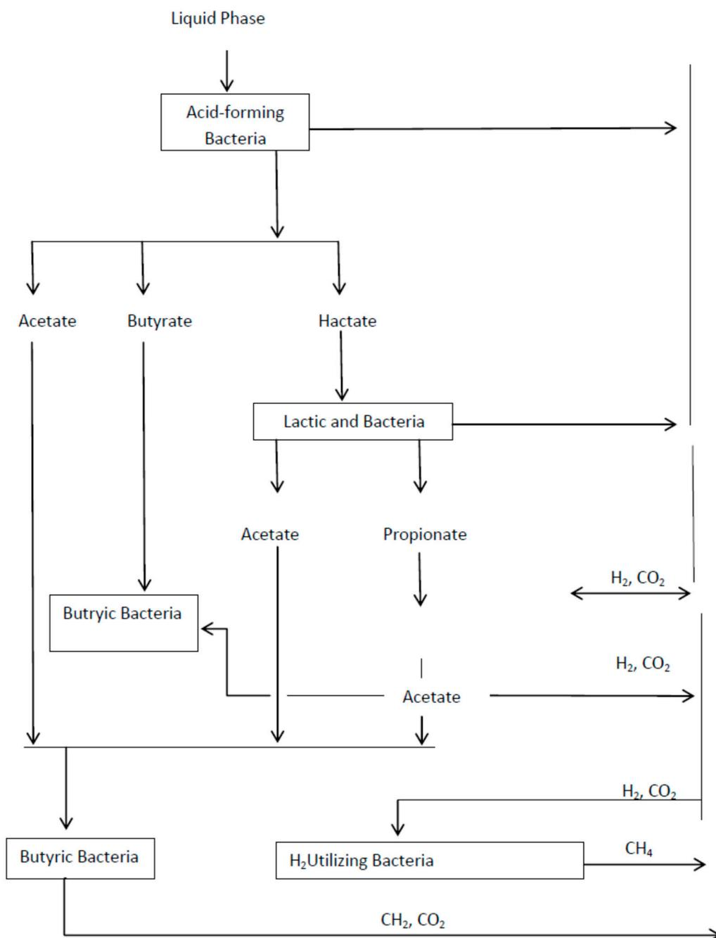
Figure 1. Schematics of the relationships between each group of bacteria in the anaerobic ecosystem.
