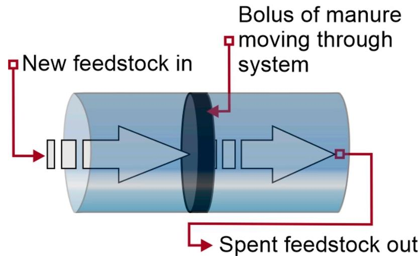
**Figure 3.** Plug-Flow Digester.
