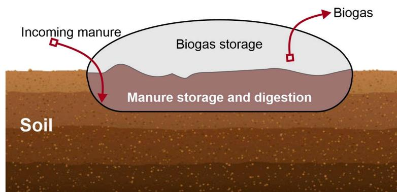
**Figure 2.** Covered Anaerobic Lagoon.
