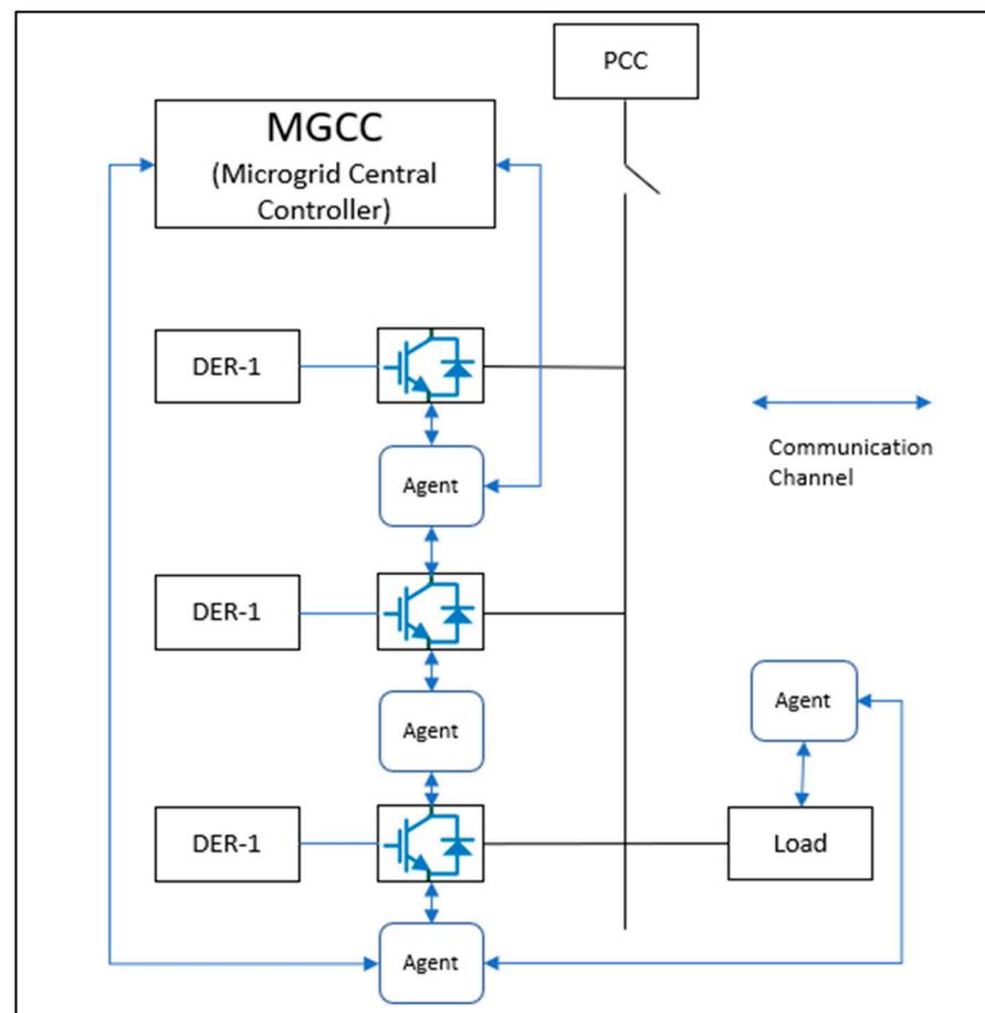
**Figure 12.** Sample architecture of multiagent control in a microgrid.
