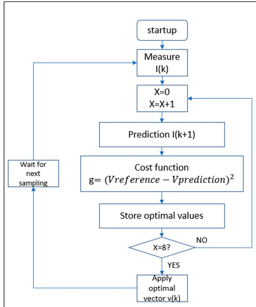
**Figure 14.** Flowchart of predictive current control.
