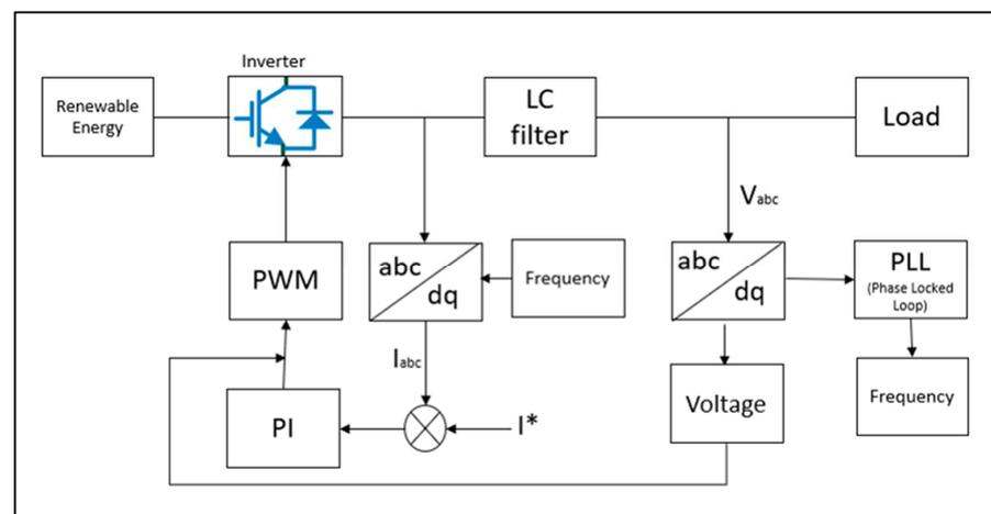
**Figure 8.** Example of  $V/f$  control strategy using  $I^*$  (reference current) in AC bus.
