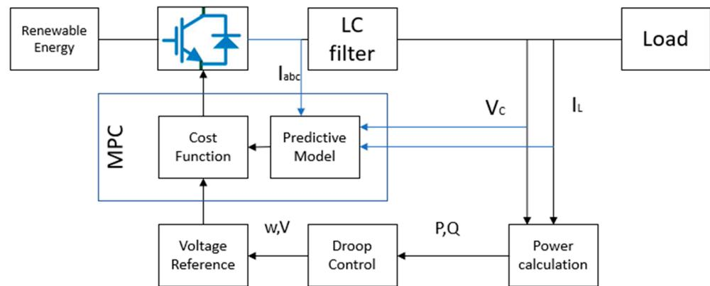
Figure 13. Typical MPC control scheme in AC MG.
