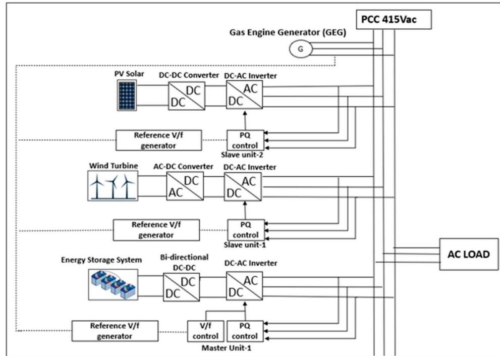
Figure 9. Sample architecture of master–slave control energy in microgrid.
