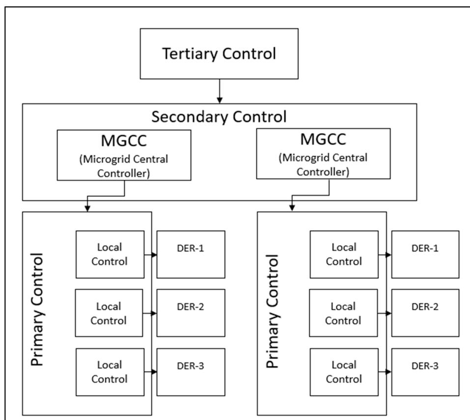
**Figure 11.** Sample architecture of hierarchical control in a microgrid.
