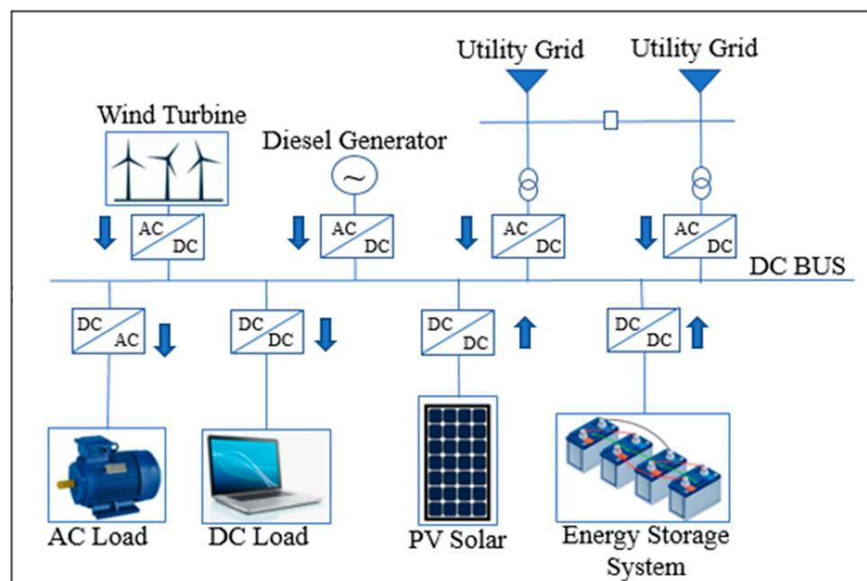
**Figure 4.** Direct current (DC) MG architecture.
