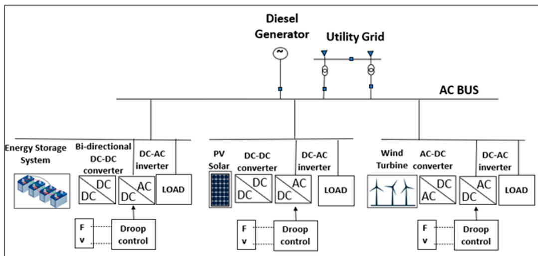
Figure 10. Sample architecture of peer-to-peer (P2P) control in microgrid.
