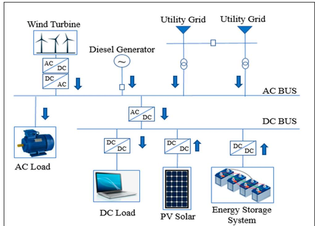
**Figure 5.** Hybrid AC/DC MG architecture.
