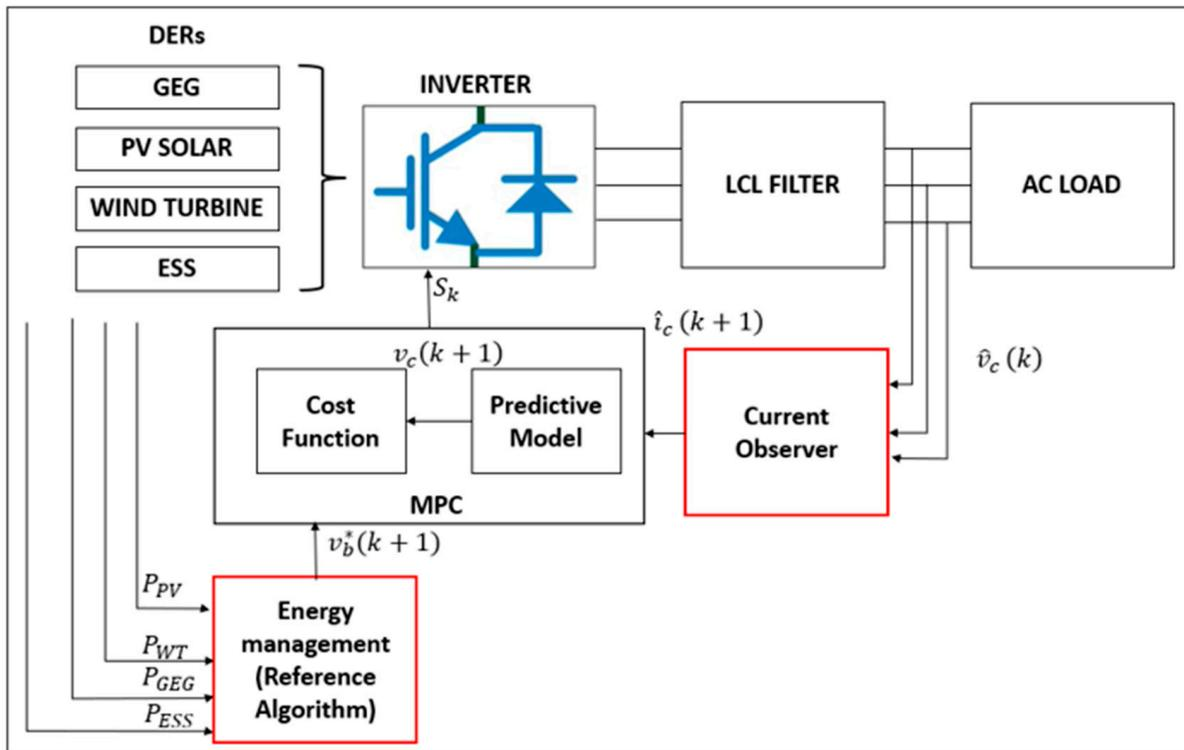
Figure 16. MPC-based EMS with the current observer.
