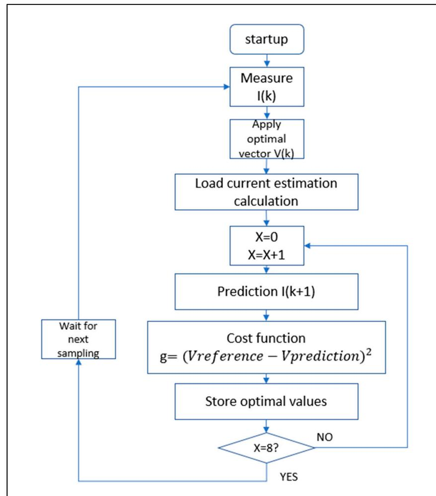
**Figure 15.** Flow chart of predictive current control with delay compensation.
