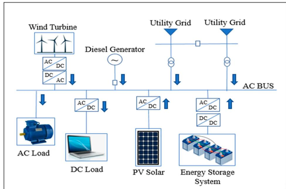
**Figure 3.** Alternative current (AC) MG architecture.
