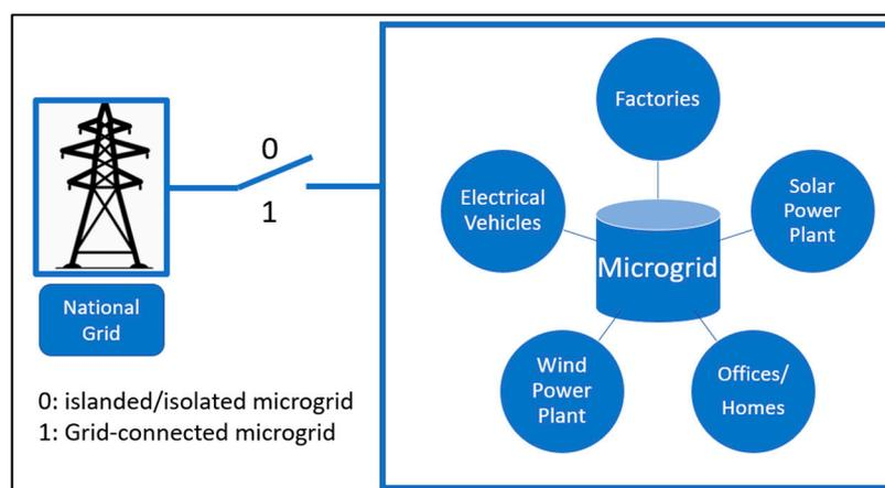
**Figure 2.** Microgrid Diagram.
