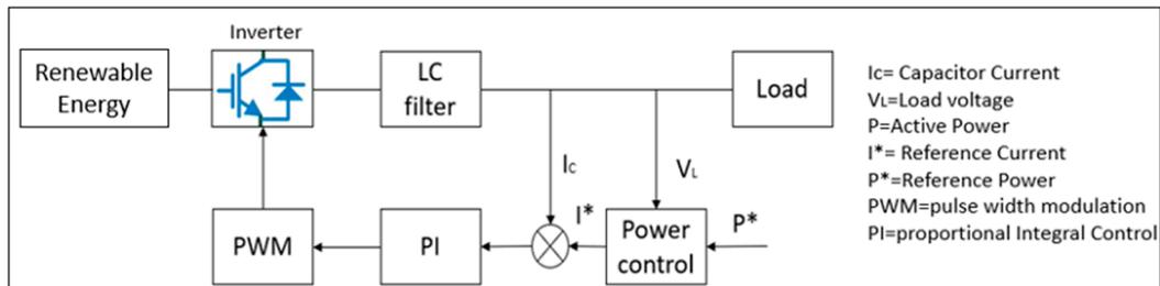
**Figure 7.** Example of constant current control with power control.
