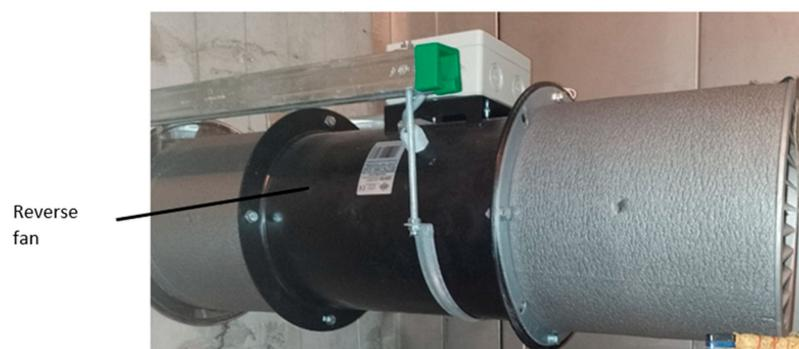
**Figure 3.** Façade ventilation unit (view from the side simulating external environment conditions).
