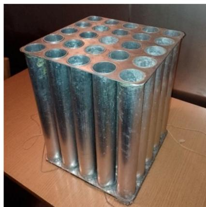
**Figure 7.** Heat exchanger 3 made of cylinders with an external diameter of 40 mm and a wall thickness of 1 mm.
