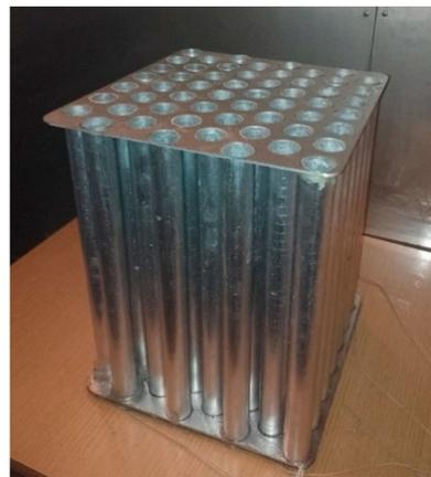
**Figure 6.** Heat exchanger 2 made of cylinders with an external diameter of 25 mm and a wall thickness of 1 mm.
