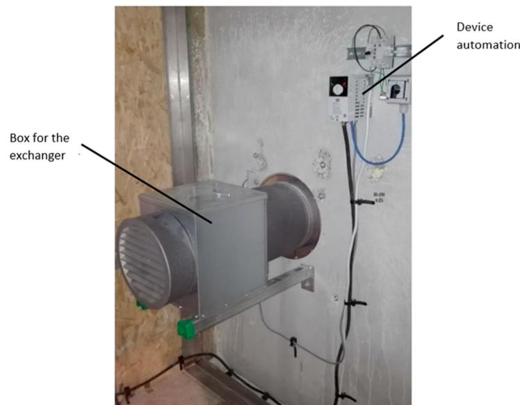
**Figure 2.** Façade ventilation unit (view from the side simulating indoor environment conditions).
