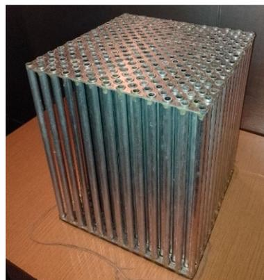
**Figure 5.** Heat exchanger 1 made of cylinders with an external diameter of 10 mm and a wall thickness of 1 mm.
