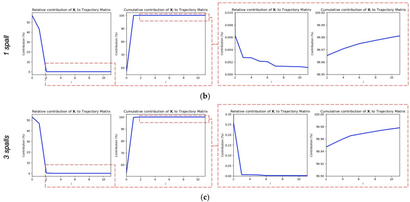
**Figure 8.** Relative and cumulative contribution of the components:  $[0, \dots, 11]$  (left),  $[2, \dots, 11]$  (right) for phase A of the bearing without faults (a), the bearing with one spall (b) and the bearing with three spalls (c).
