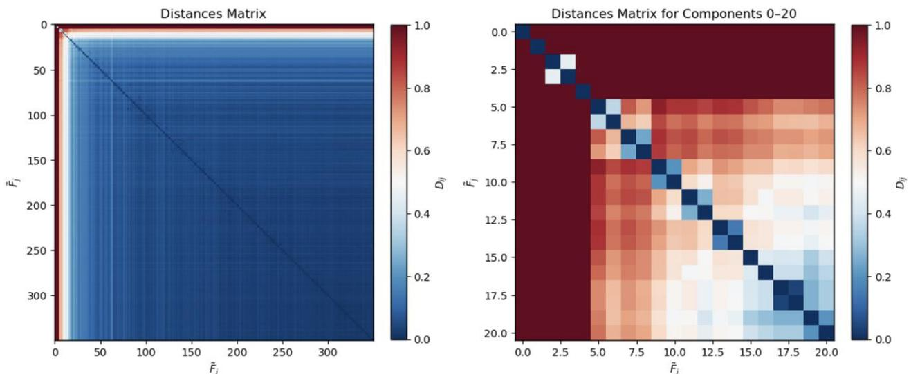
**Figure 9.** Distance matrix based on the Frobenius norm for phase A of the bearing without faults, on the left for the complete set of components (350) and on the right for the investigated set of informative components (20).
