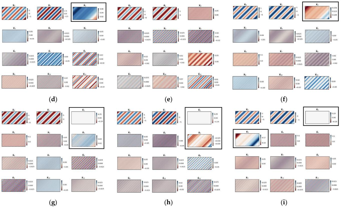
**Figure 7.** Comparison of the trajectory matrix decomposition of all signals in consideration: bearing without faults (a–c); the bearing with one spall (d–f); the bearing with three spalls (g–i); phase A (a,d,g); phase B (b,e,h); phase C (c,f,i).
