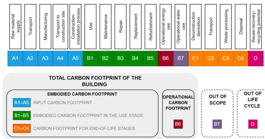
**Figure 1.** Types of carbon footprint from the perspective of a building structure. Own elaboration based on.
