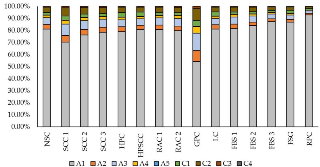
**Figure 10.** Percentage contribution of the different life cycle phases of the analyzed concretes to the carbon footprint value.
