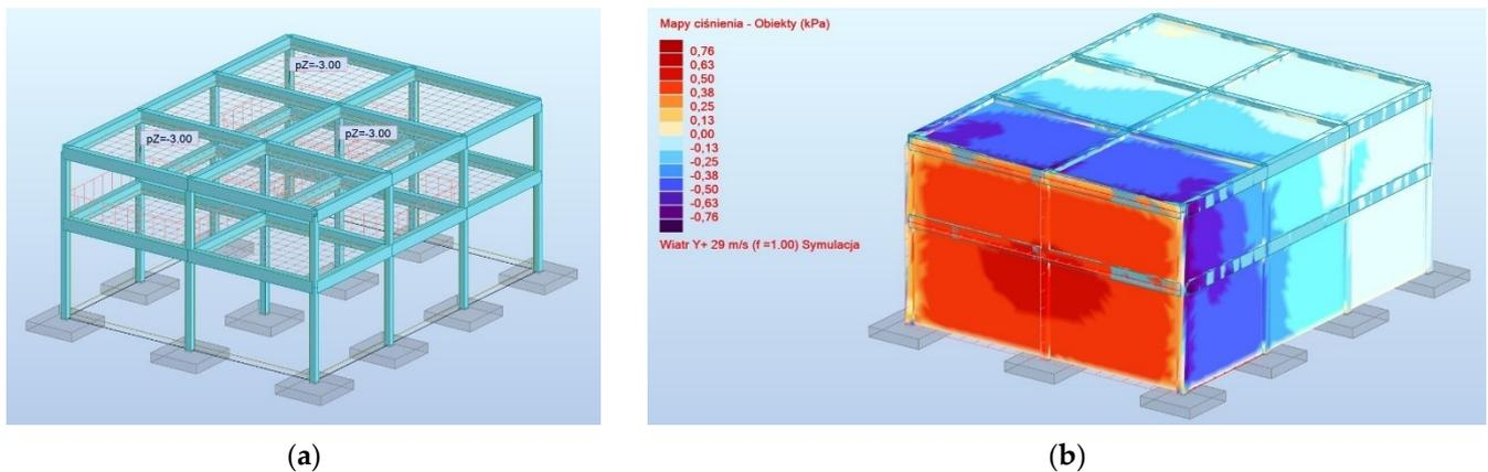
**Figure 5.** An exemplary load acting on the analyzed reinforced concrete structure: (a) example service load; (b) example wind load (push on gable wall).
