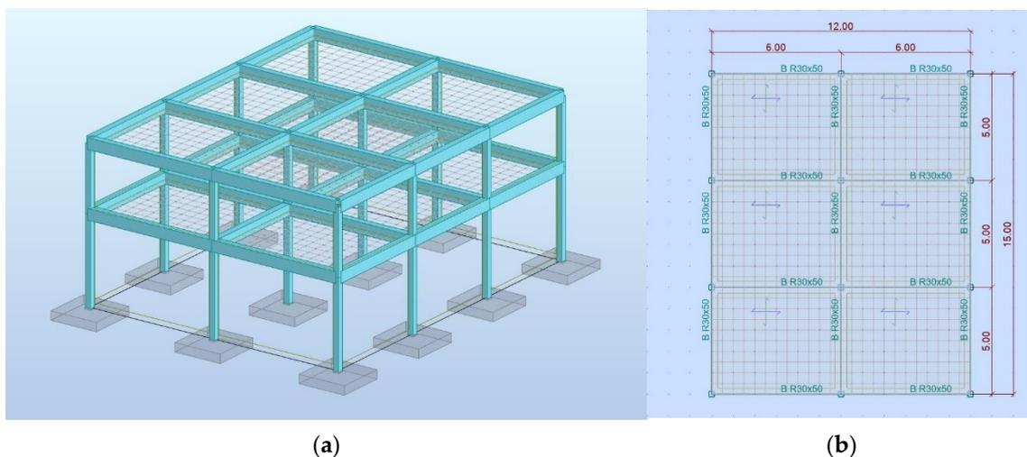
**Figure 4.** Reinforced concrete structure model under analysis: (a) general view; (b) view of the reinforced concrete structure (geometric dimensions in m).
