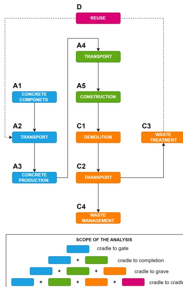
Figure 2. Life cycle of concrete. Own elaboration based on [14,15].
