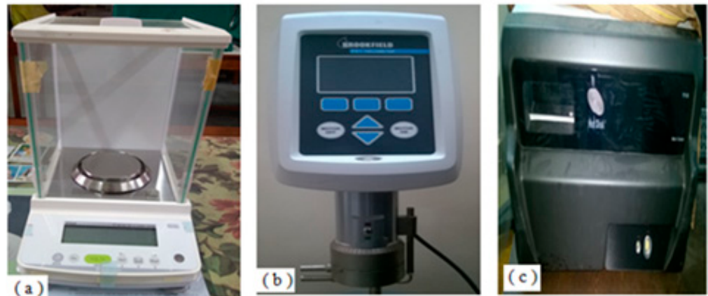
Figure 4. Photographs of (a) digital weighing balance, (b) Brookfield DV1 digital viscometer, and (c) hot disc thermal constant analyzer apparatus [48].
