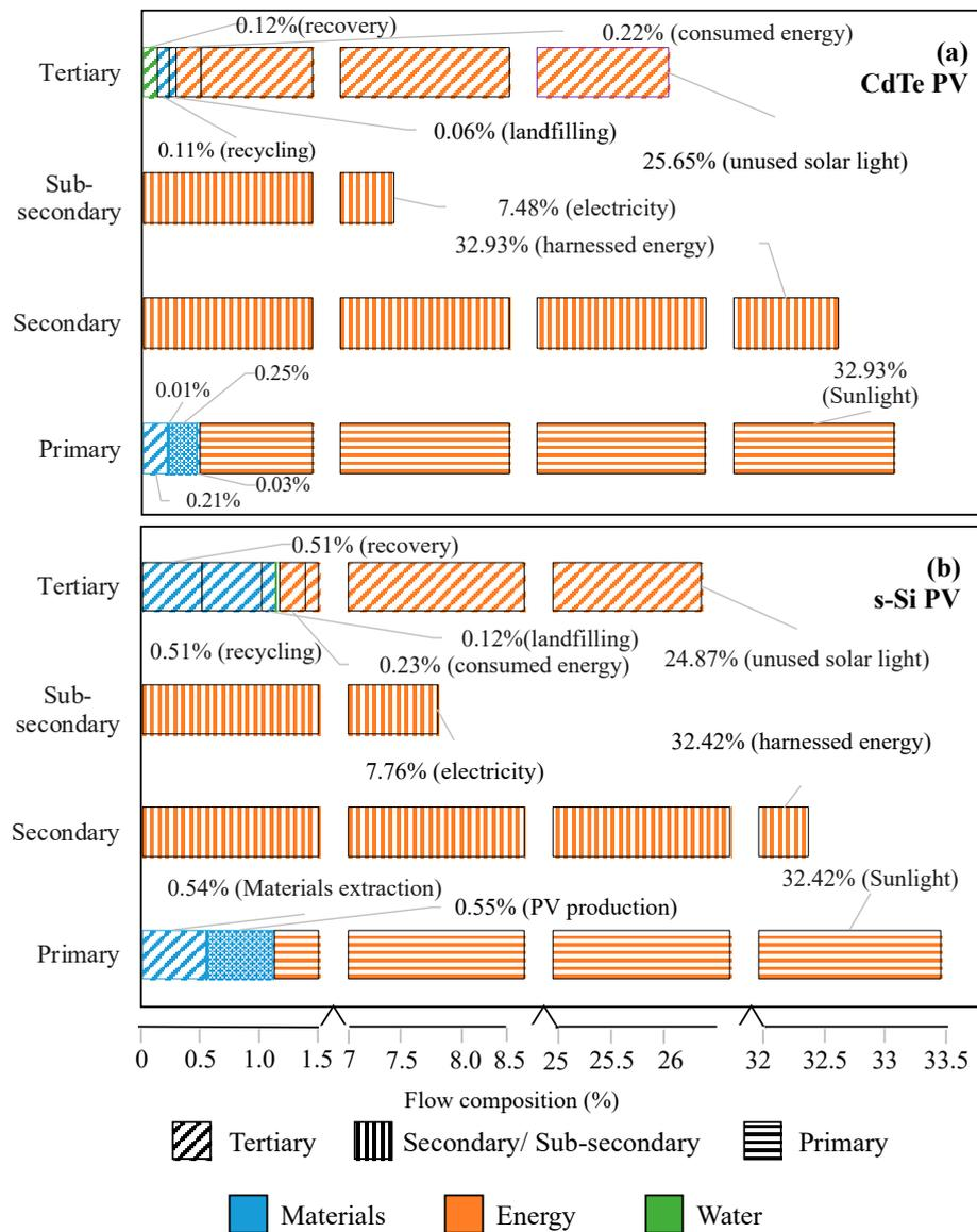
Figure 2. MEW flow of the CdTe (a) and s-Si (b) PV technology. The trophic characteristics are shown for their percentage of the total inflow in each industry.
