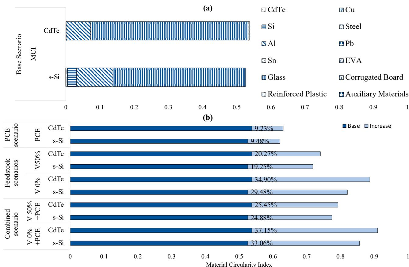
**Figure 3.** MCIs of CdTe and s-Si solar panels: (a) the impact of each PV component to the MCI metric, and (b) the impact of alternative scenarios, including the changed in PCE, virgin feedstock rates and their combinations on MCI metric. The increment (%) for each scenario is also shown with transparent bars in (b).
