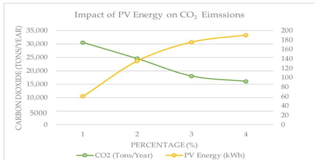
Figure 10. Impact of PV Energy Penetration on CO<sub>2</sub>.
