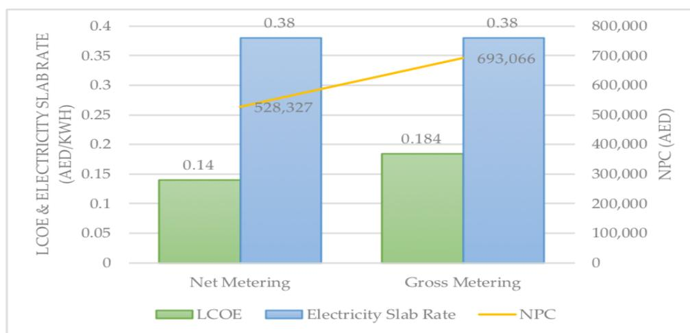
Figure 8. Cost Characteristics of Grid-Connected PV System.
