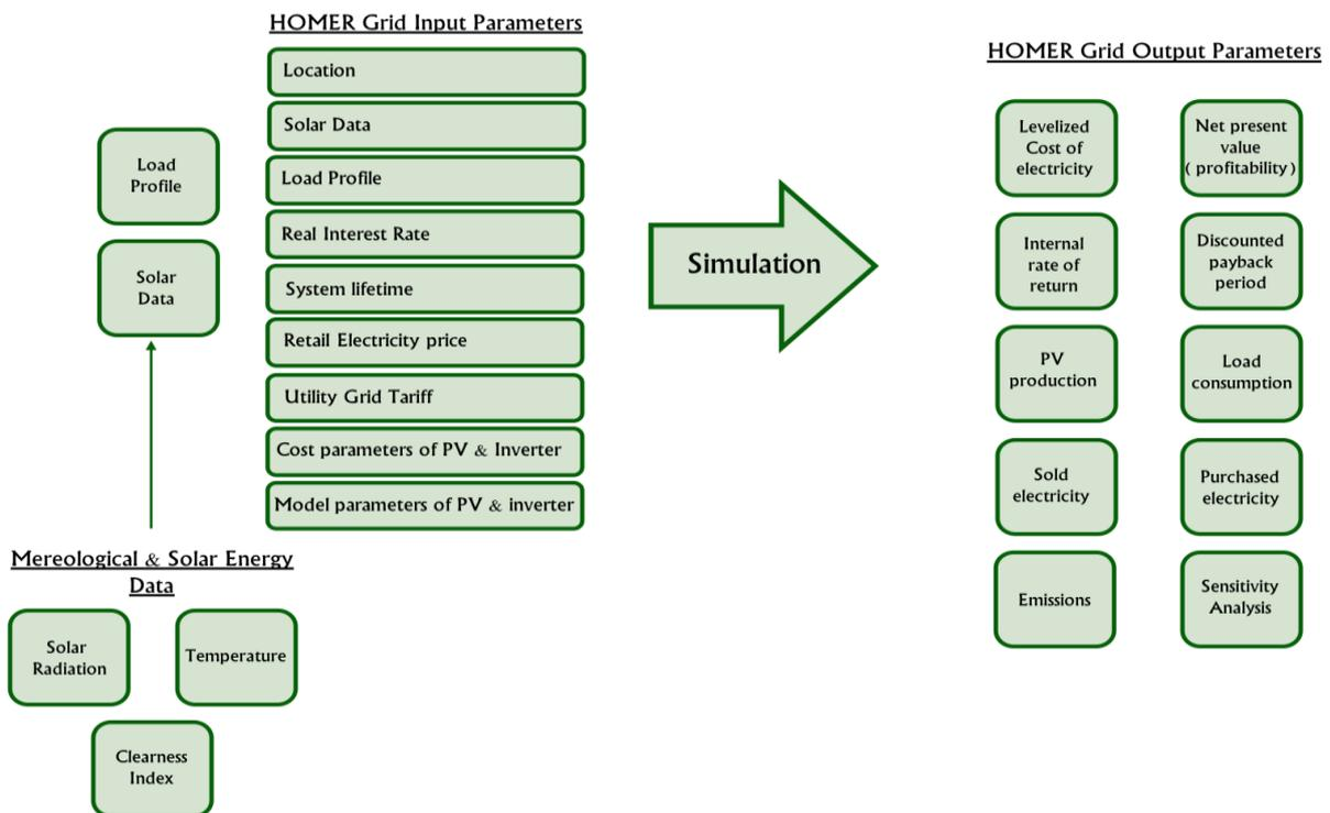
**Figure 2.** HOMER Grid Schematic Diagram.
