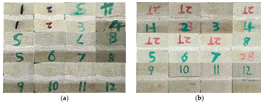
Figure 9. The completed direct shear experiment sample. (a) is shear type experimental sample; (b) is a tensile type experimental sample.
