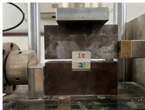
Figure 10. Fault rocks placed in the RJST-616 direct shear apparatus.
