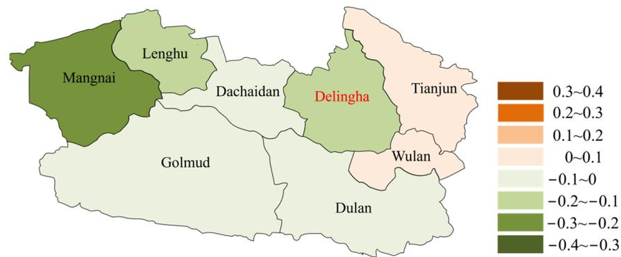
**Figure 2.** The Kendall correlation coefficient of wind and solar in Haixi.
