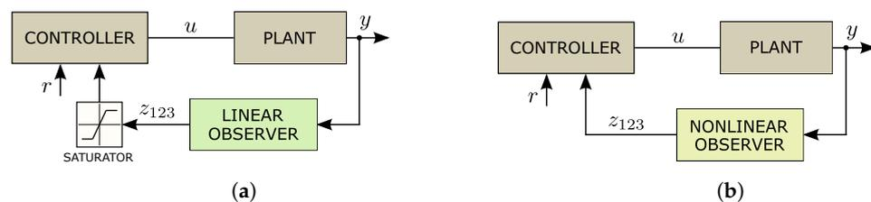
Figure 9. Block diagrams of the implemented controllers. (a) Linear ADRC. (b) Nonlinear ADRC.
