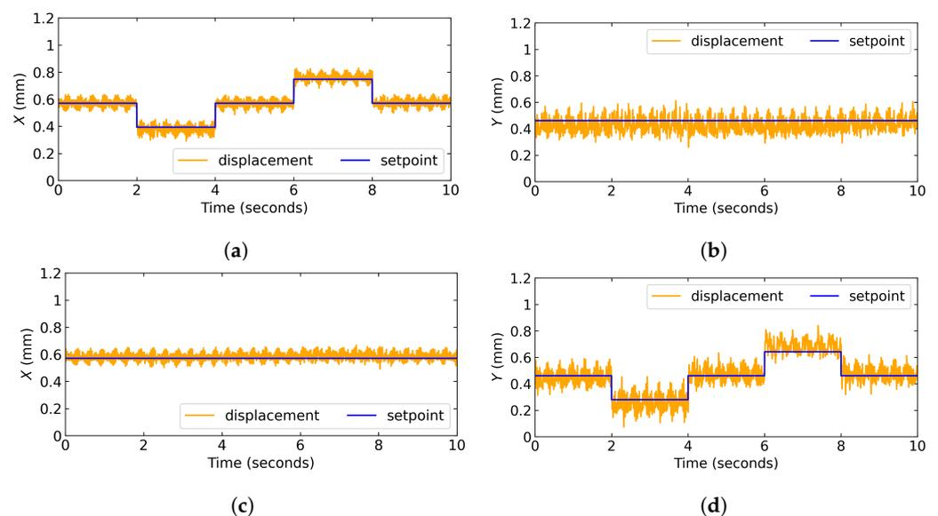
**Figure 15.** Response of radial position control under step setpoint changes for Linear ADRC. (a) X-axis behavior with step setpoint changes applied. (b) Y-axis behavior with step setpoint changes applied to X-axis. (c) X-axis behavior with step setpoint changes applied to Y-axis. (d) Y-axis behavior with step setpoint changes applied.
