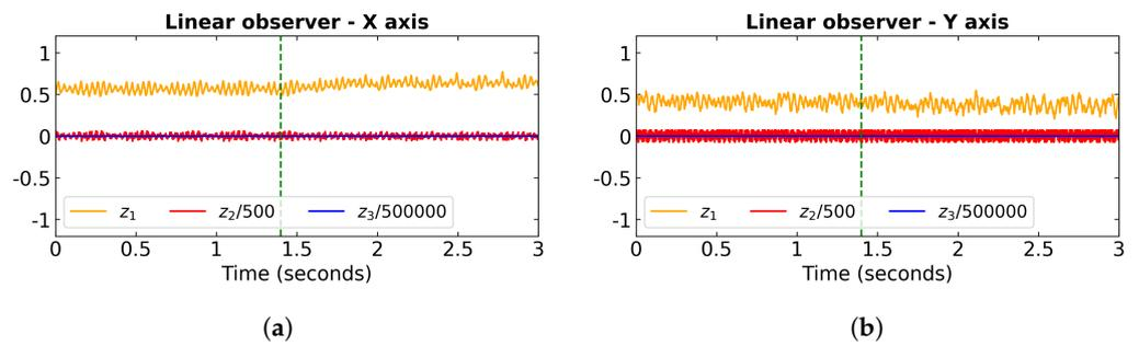
**Figure 18.** Estimated states behavior for linear ADRC under radial load application. (a) Linear ADRC—X-axis states. (b) Linear ADRC—Y-axis states.
