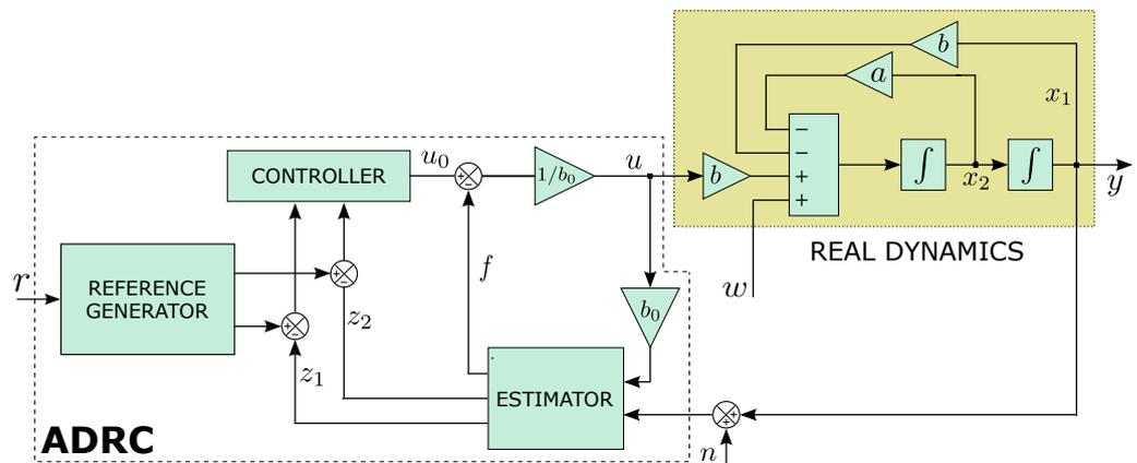
Figure 6. ADRC block diagram of a generic second order plant.
