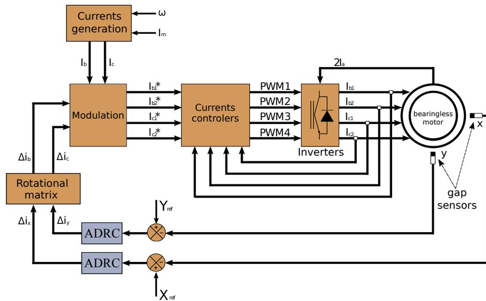
Figure 13. Control system diagram.
