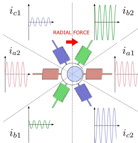
**Figure 4.** Stator of the bearingless induction motor with split-winding subjected to right-side radial force.
