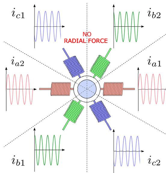
**Figure 3.** Stator of the bearingless induction motor with split winding.
