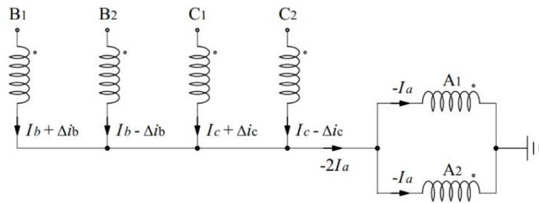
**Figure 2.** Connection of the coils for two-phase position control.
