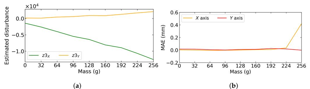
**Figure 20.** Generalized disturbance estimation and mean steady state error for X and Y axes to different values of radial load aligned with the X-axis. (a) Generalized disturbance estimation ( $z_3$ ). (b) Mean absolute error for X and Y axes.
