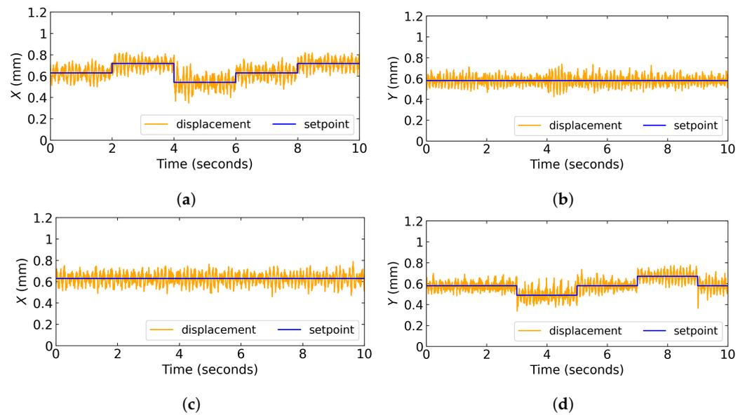
**Figure 16.** Response of radial position control under step setpoint changes for Nonlinear ADRC. (a) X-axis behavior with step setpoint changes applied. (b) Y-axis behavior with step setpoint changes applied to X-axis. (c) X-axis behavior with step setpoint changes applied to Y-axis. (d) Y-axis behavior with step setpoint changes applied.
