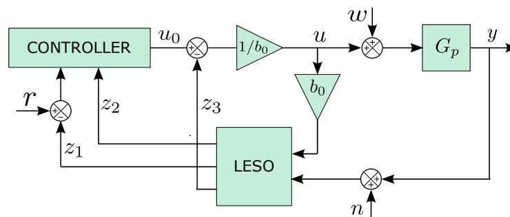
Figure 8. LADRC block diagram.
