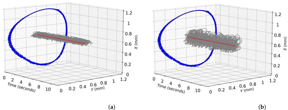
**Figure 14.** Steady state response of radial position control for the linear and nonlinear controllers in 3D. (a) Linear ADRC. (b) Nonlinear ADRC.
