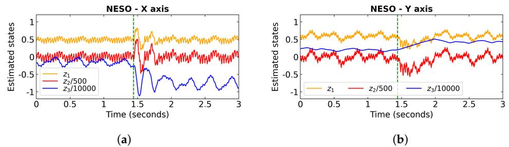
**Figure 19.** Estimated states behavior for nonlinear ADRC under radial load application. (a) Nonlinear ADRC—X-axis states. (b) Nonlinear ADRC—Y-axis states.
