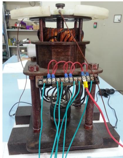
**Figure 12.** Split-winding bearing machine prototype.
