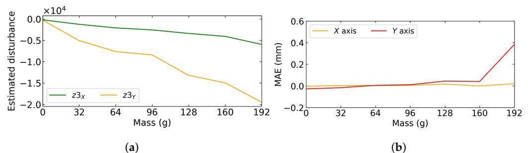
**Figure 21.** Generalized disturbance estimation and mean steady state error for X and Y axes to different values of radial load aligned with the Y-axis. (a) Generalized disturbance estimation ( $z_3$ ). (b) Mean absolute error for X and Y axes.
