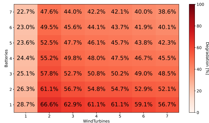
Figure 27. Degradation of the batteries over 20 years of usage with strategy 4.
