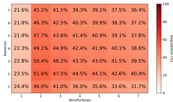
Figure 26. Degradation of the batteries over 20 years of usage with strategy 3.
