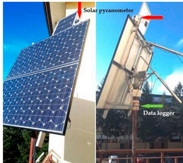
**Figure 3.** PV panels with an integrated tracking system. Position of the solar irradiance monitoring system (SPN1) and data logger module (GP1).
