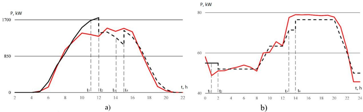
**Figure 2.** Correction of the forecast generation schedule of PV (a) and WPPs (b).
