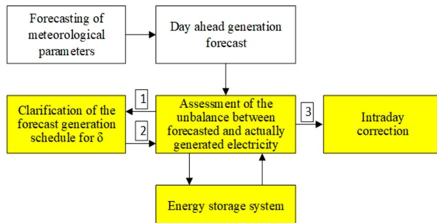
**Figure 1.** Structural diagram of the reduction of electricity imbalance in EPS with RES.
