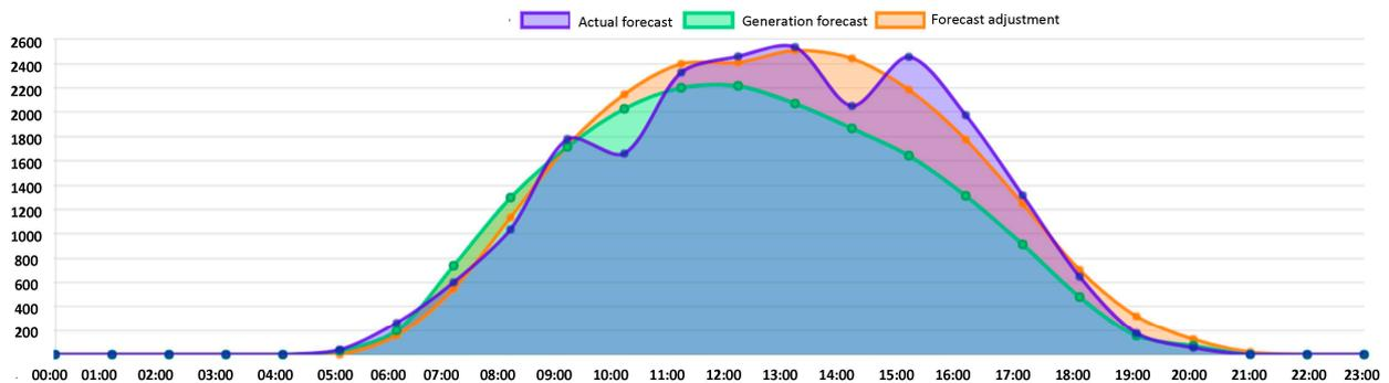
Figure 4. Correction of PV generation forecasting based on the results of error control.
