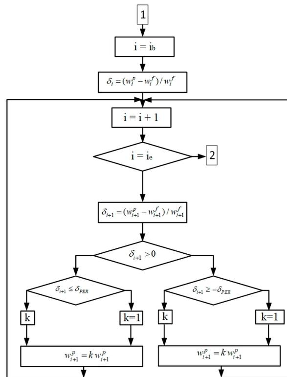
Figure 3. Algorithm of the program for the hourly correction of forecasting the power generation by PV.
