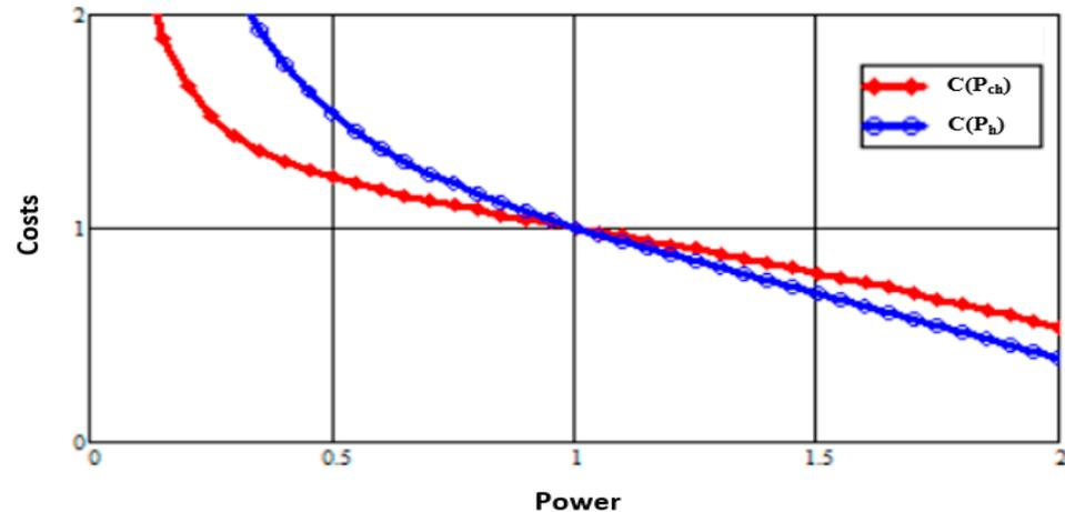
**Figure 5.** Sensitivity of relative costs to changes in the power generation of biogas (red curve) and to changes in the power generation of hydrogen technologies (blue curve).
