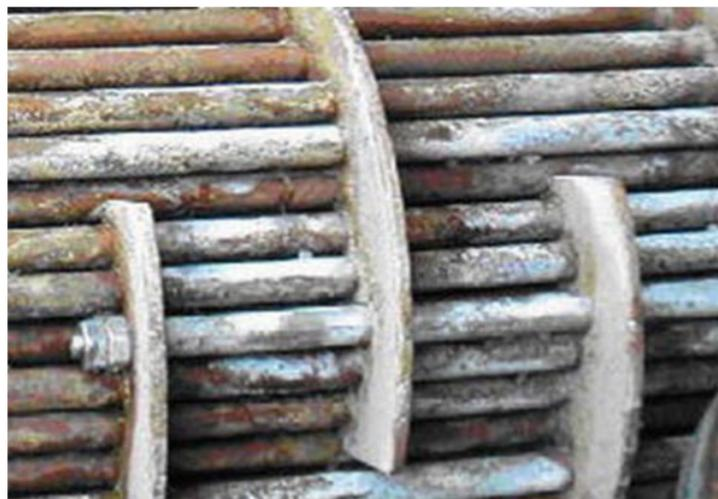
**Figure 3.** Accumulation of precipitated salts in heat exchanger tubes [4].
