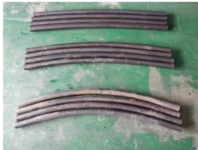
Figure 4. Coiled tubing with different radii of curvature.
