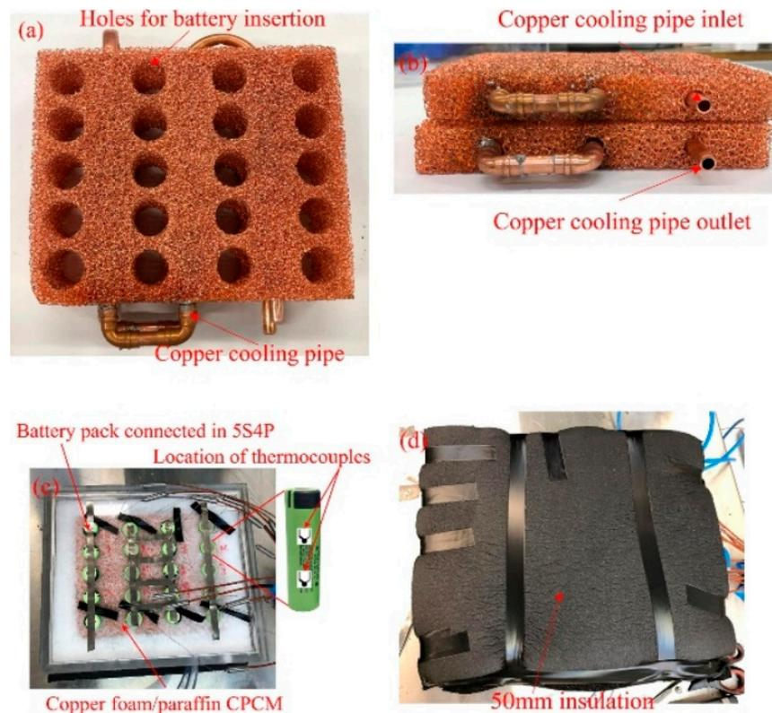
**Figure 21.** The hybrid active-passive BTMS described in [74]. (a) the Cu MF and the cooling pipes embedded into it—top view; (b) same as (a), front view; (c) PCM-impregnated Cu foam; (d) BTMS with insulation applied.
