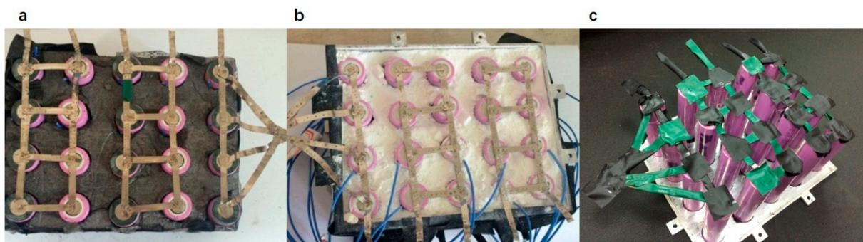
**Figure 2.** Li-ion battery packs: (a)—60 wt% RT44HC/EG; (b)—60 wt% RT44HC/fumed silica; (c)—no PCM. Reproduced from [34] with permission from Elsevier.
