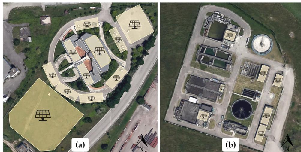
**Figure 3.** Aerial view of the surfaces selected for installing the PV plant, belonging to  $Us\#1$  (a) and  $Us\#2$  (b).
