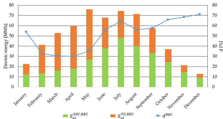
**Figure 10.** Producibility of the PV plant serving  $Us\#1$  and  $Us\#2$  in the REC scenario. Electric energy virtually shared and fed to the grid and self-consumption index in 2021.
