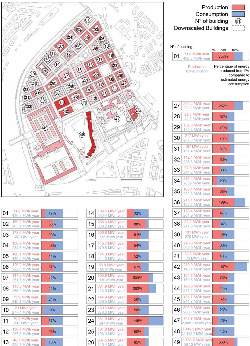
Figure 16. Testaccio\_Electricity production map of actual scenario estimated through PVGIS for each building.
