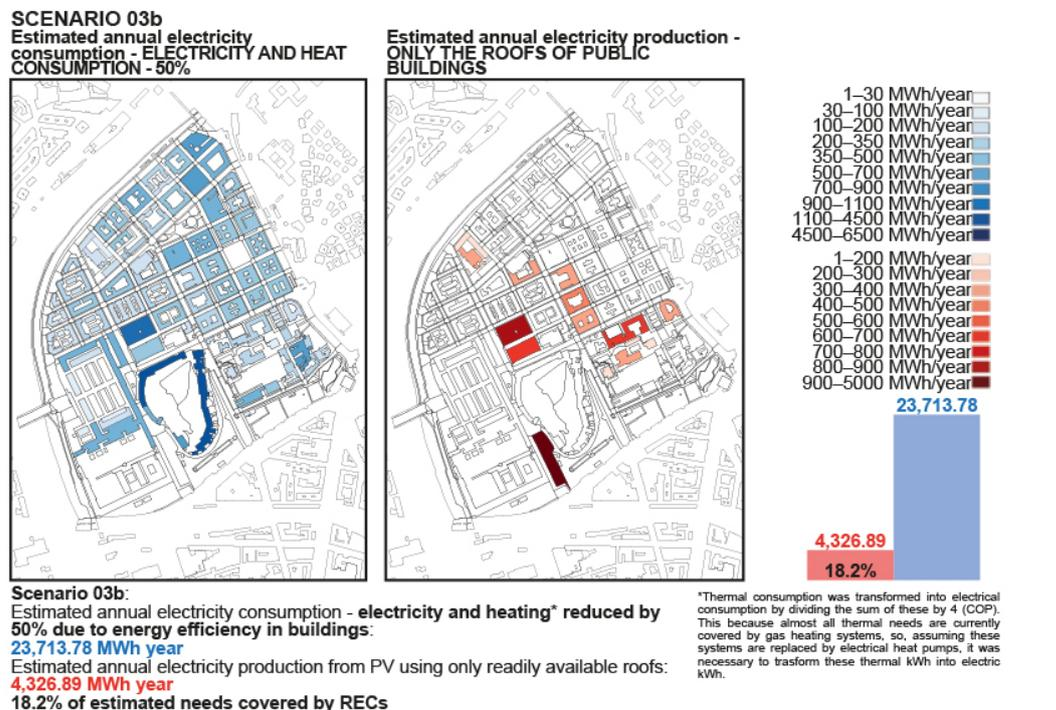
**Figure 10.** Testaccio\_Scenario 03b—Estimated consumption (reduction of 50%) and production (using only the roofs of public buildings).
