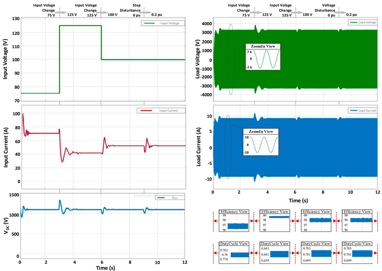
**Figure 7.** Performance results under varying input voltages and input disturbances.
