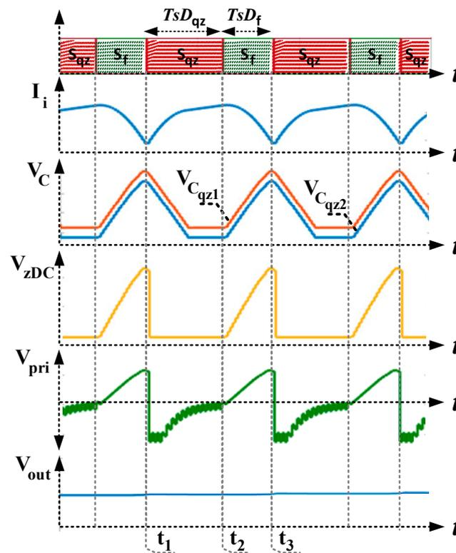
Figure 4. Key waveforms of the qZ\_iFC.
