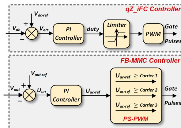
Figure 3. Control scheme of the proposed system.
