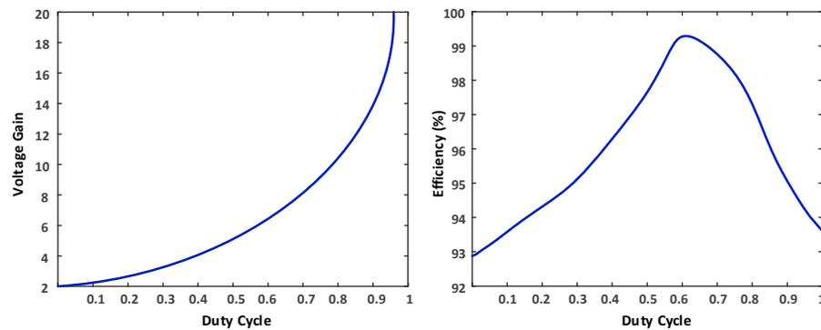
Figure 2. Voltage gain and efficiency curve of the proposed qZ\_iFC.
