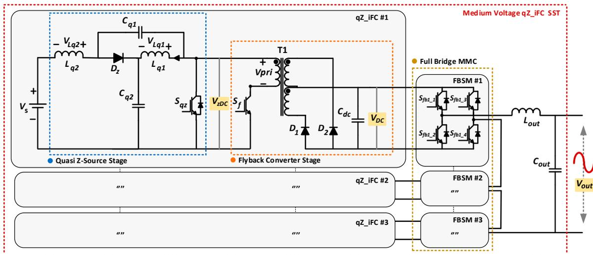
Figure 1. Circuit diagram of novel qZ\_iFC-based SST.
