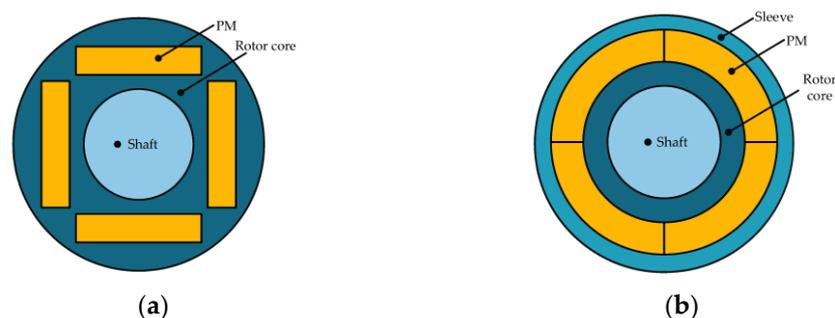
**Figure 6.** Schematic representation of permanent magnet synchronous motor structure with (a) interior rotor; (b) exterior or surface rotor layout; with windings and air gaps, replicated from [58].
