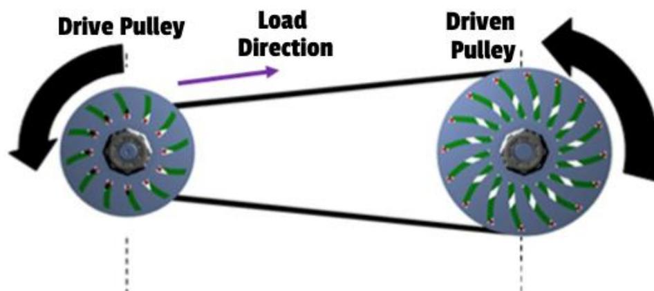
**Figure 9.** CVT operation principle, currently implemented at most hybrid or battery electric vehicles and electric scooters [76].
