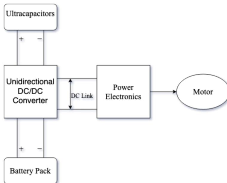
**Figure 11.** Common topology for the hybrid energy system consisting of batteries and ultracapacitors.
