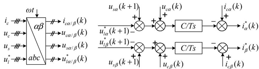
Figure 3. Reference current generation mechanism based on DBDC.
