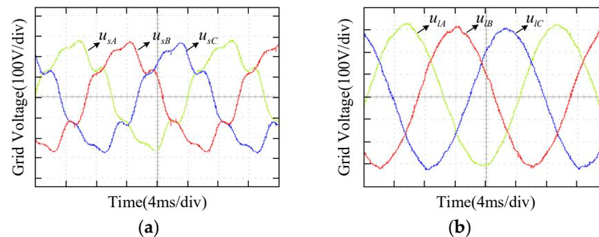
**Figure 16.** Temporary sag and harmonic conditions. (a) Grid voltage before compensation; (b) load voltage after compensation.
