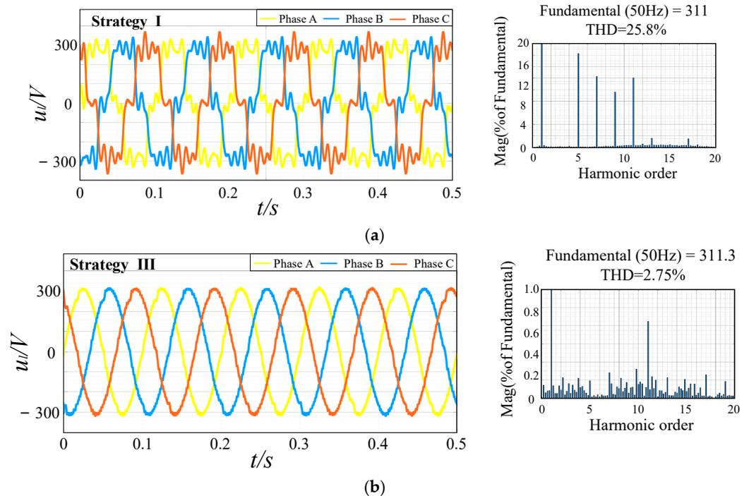
**Figure 13.** Load voltage after compensation of harmonics of different frequencies. (a) Load voltage after compensation of the 9th and 11th harmonics via Strategy I; (b) load voltage after compensation of the 9th and 11th harmonics via Strategy III.
