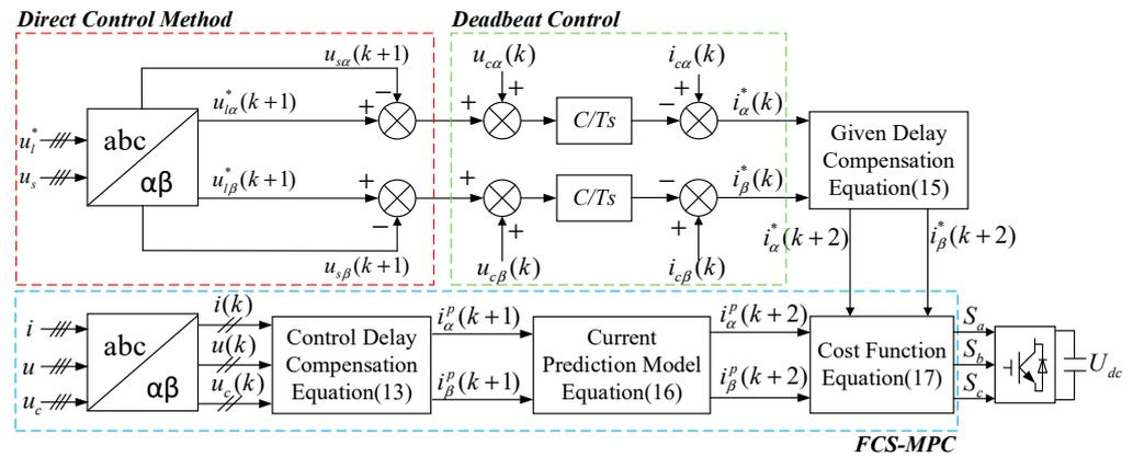
Figure 5. Control block diagram of SAPF system based on the DBDC-FCS-MPC strategy.
