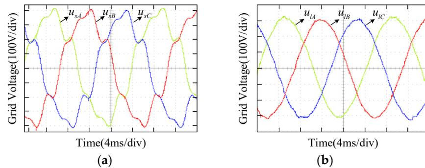
**Figure 15.** Temporary swell and harmonic conditions. (a) Grid voltage before compensation; (b) load voltage after compensation.
