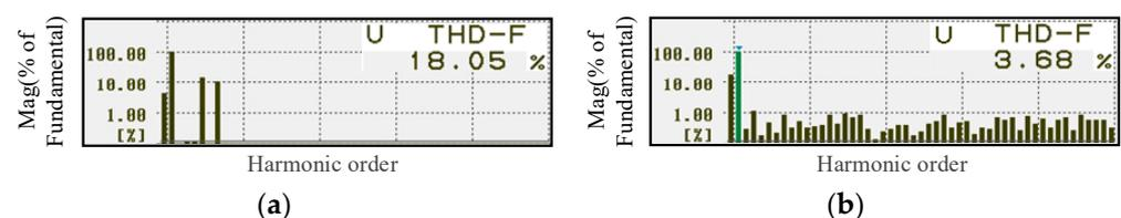
**Figure 17.** The THD rate of voltage based on Strategy III. (a) Grid voltage before compensation; (b) load voltage after compensation.
