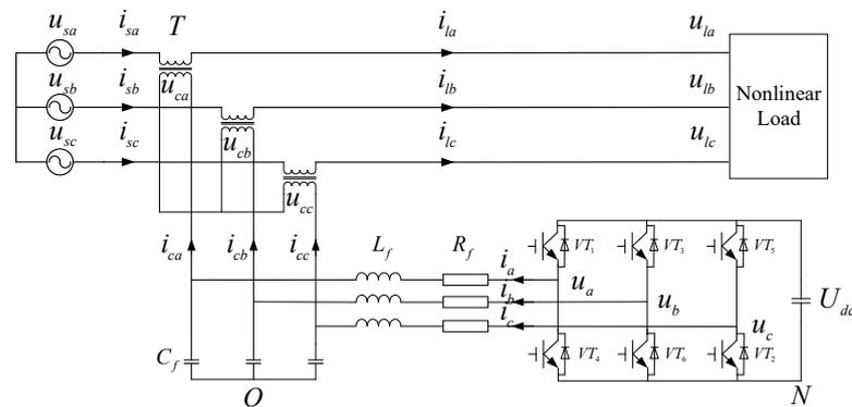
Figure 1. Three-phase two-level SAPF topology.
