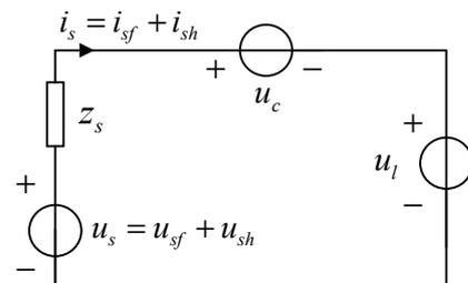
Figure 2. SAPF single-phase equivalent circuit diagram.
