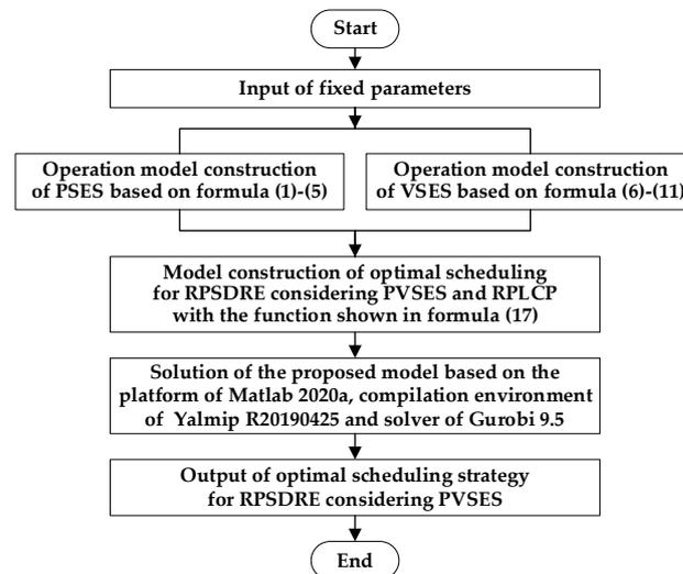
Figure 2. Flowchart of optimal scheduling for the RPSDRE considering PVSES.
