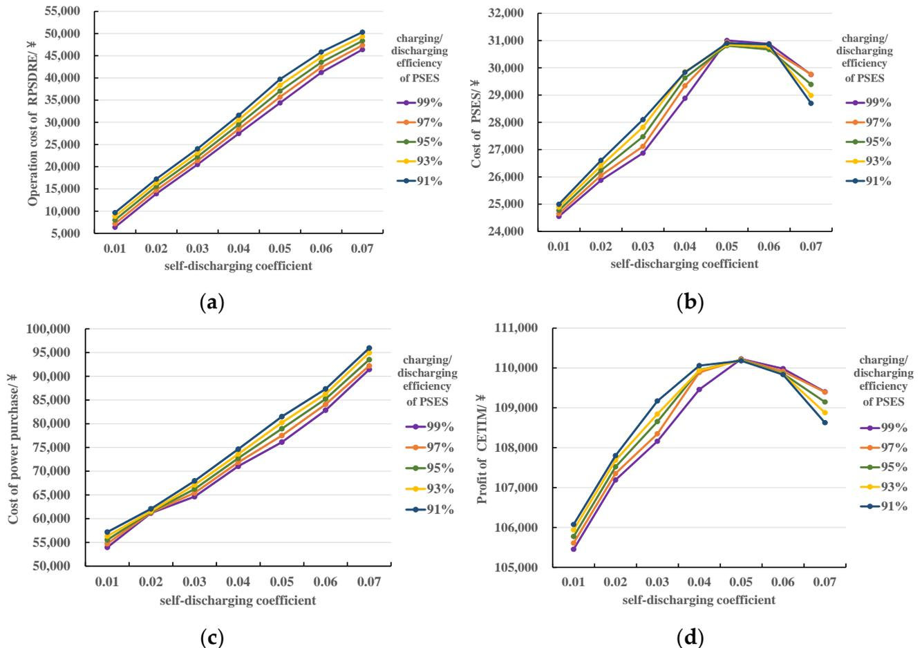
**Figure 5.** Optimal scheduling results of the RPSDRE considering the degradation of battery PSES: (a) operational cost of the RPSDRE; (b) cost of PSES; (c) cost of power purchase from the superior grid; and (d) profit of CETIM.
