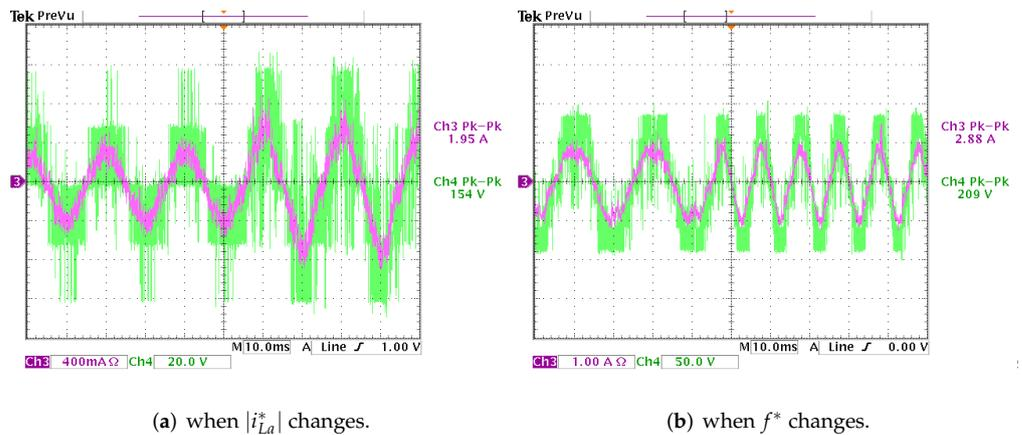
Figure 9. Load current and CHB output voltage in transient conditions.
