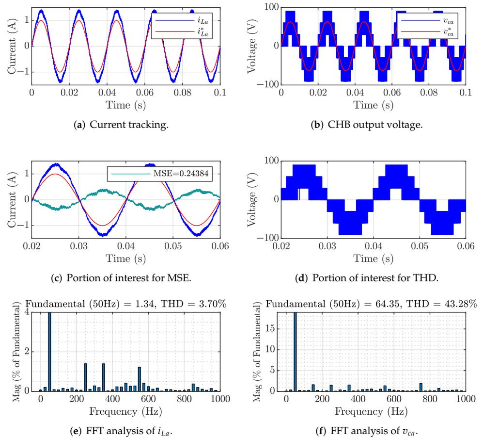
**Figure 5.** Simulation results for phase *a* in the presence of parametric uncertainties.
