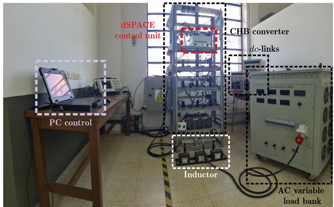
**Figure 6.** Experimental test equipment.
