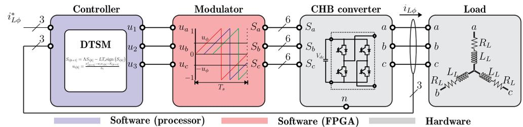
Figure 2. Block diagram of the DTSM current control method.
