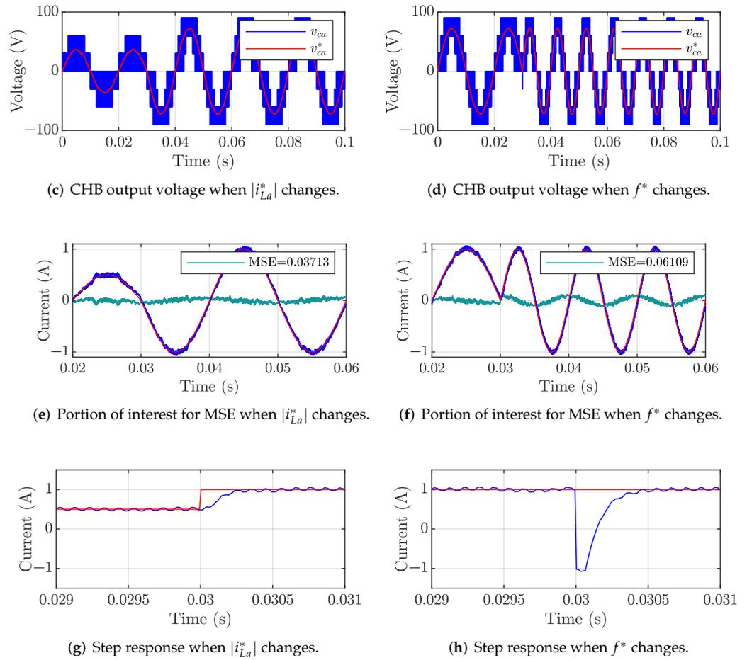
Figure 4. Simulation results for phase  $a$  (a–f) and  $i_{Ld}$  (g,h), in transient conditions.
