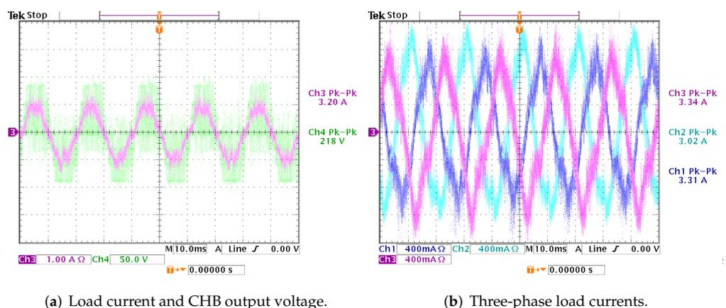
Figure 11. Load currents and CHB output voltage in the presence of parametric uncertainties.
