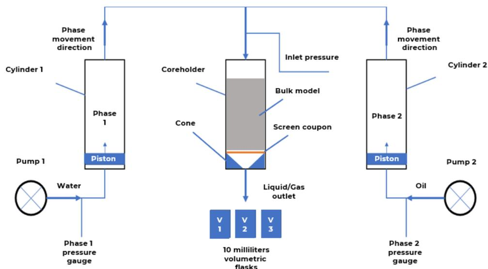
**Figure 5.** Scheme of the installation for Prepack SRT implementation [by authors].
