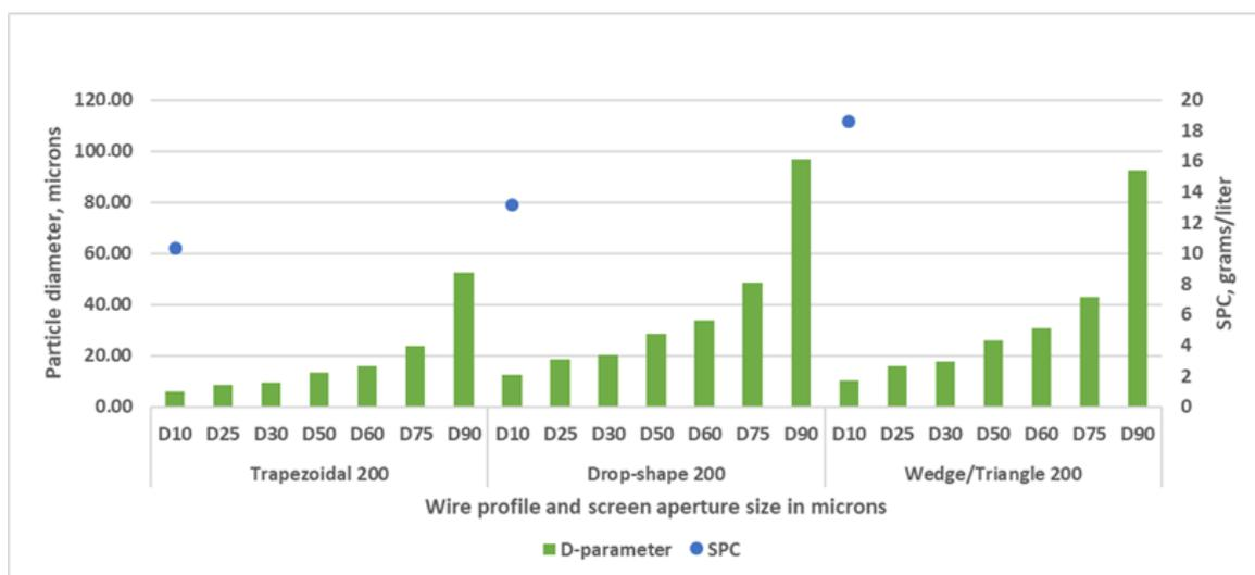
Figure 7. Experimental results for screens with an aperture size of 200 microns.
