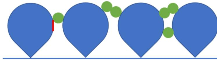
**Figure 12.** Drop-shaped wire profile and its interaction with particles.
