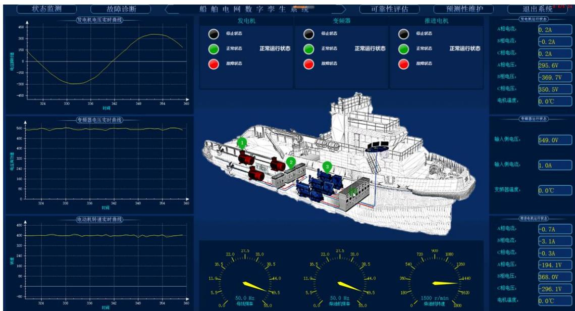
**Figure 14.** DT software platform of an all-electric smart vessel power system.
