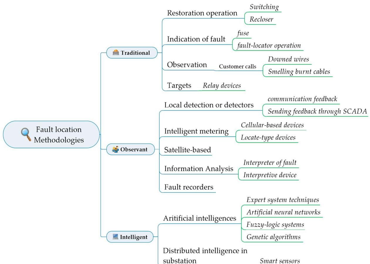
Figure 6. Fault location Methodologies for power systems [70].
