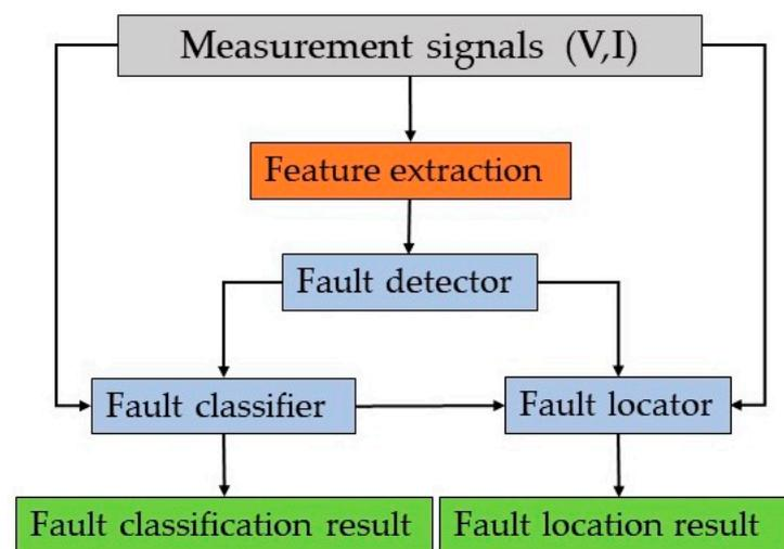
**Figure 7.** Fault location, classification, detection framework [73].
