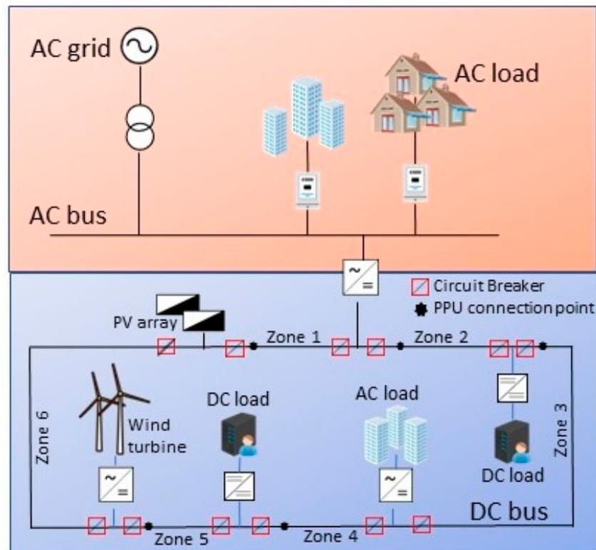
**Figure 13.** Schematic diagram of low-voltage DCMG with PPU units [124].
