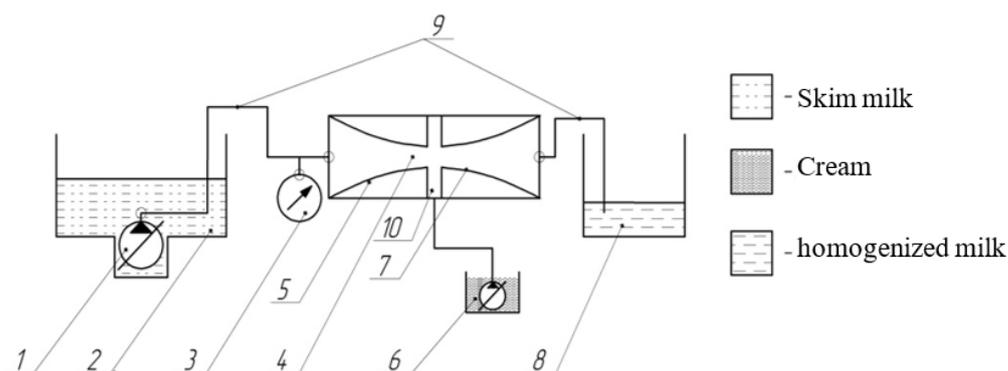
**Figure 2.** Technological scheme of the homogenizer for dispersing the fat phase of milk emulsion: 1—gear pump for supplying skim milk; 2—container for skim milk; 3—manometer; 4—place of greatest narrowing; 5—inner surfaces of the confusor; 6—gear pump for supplying cream; 7—inner surfaces of the diffuser; 8—container for draining the processed product; 9—flexible pipelines; and 10—ring slot for feeding the fatty phase.
