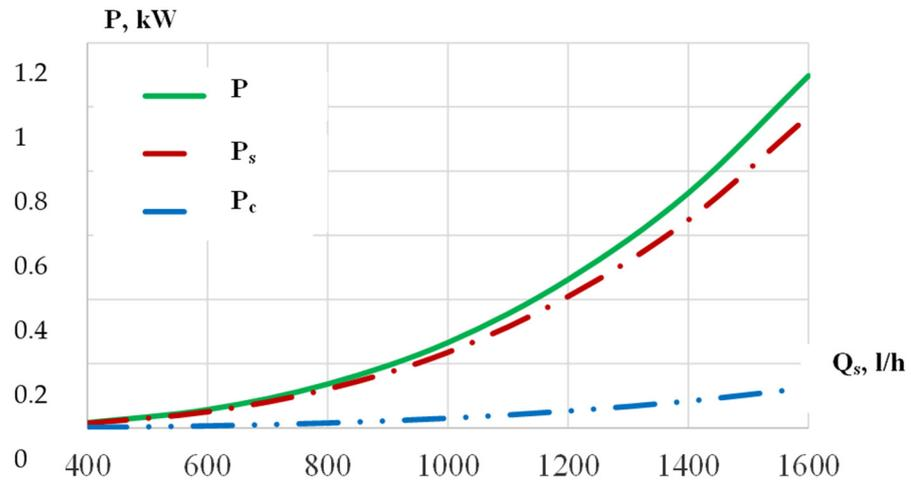
**Figure 4.** Dependence of the capacity of the cream, skim milk supply pumps and the total capacity of the JSHMSSFP  $P_c$ ,  $P_s$ , and  $P$  on the supply of skim milk  $Q_s$  (at  $d_k = 3$  mm;  $\mu_k = 0.95$ ;  $F_n = 3.5\%$ ;  $F_s = 0.05\%$ ;  $F_c = 40\%$ ;  $h = 0.6$  mm;  $\mu_B = 0.3$ ).
