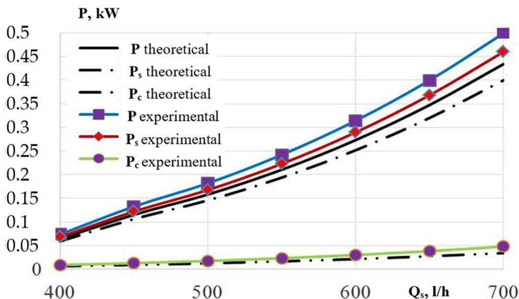
**Figure 6.** Graph of the dependence of the capacity of pumps for supplying skim milk, cream, and total capacity on the performance of the jet-slot milk homogenizer.
