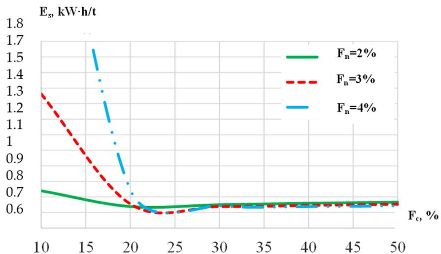
**Figure 5.** Dependence of the specific energy consumption  $E_s$  on the fat content of cream  $F_c$  and normalized milk  $F_n$  (at  $d_k = 3$  mm;  $F_s = 0.05\%$ ;  $h = 0.5$  mm;  $\mu_B = 0.3$ ;  $Q = 1000$  kg/h,  $\mu_k = 0.98$ ).
