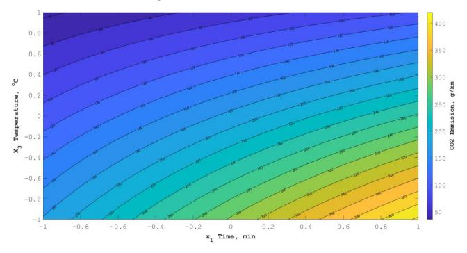
**Figure 15.** Change of CO<sub>2</sub> emissions depending on the variability of factors  $x_1$  and  $x_3$  for a vehicle (EV) covering a distance of 3 km ( $x_2 = 0$ ).
