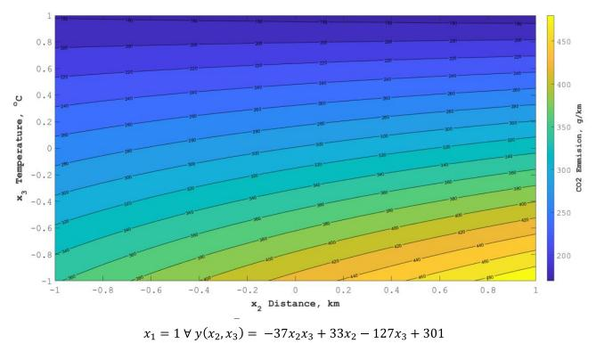
**Figure 4.** Change in CO<sub>2</sub> emissions depending on the variability of factors  $x_2$  and  $x_3$  for a vehicle (ICE) moving for 10 min ( $x_1 = 1$ ).
