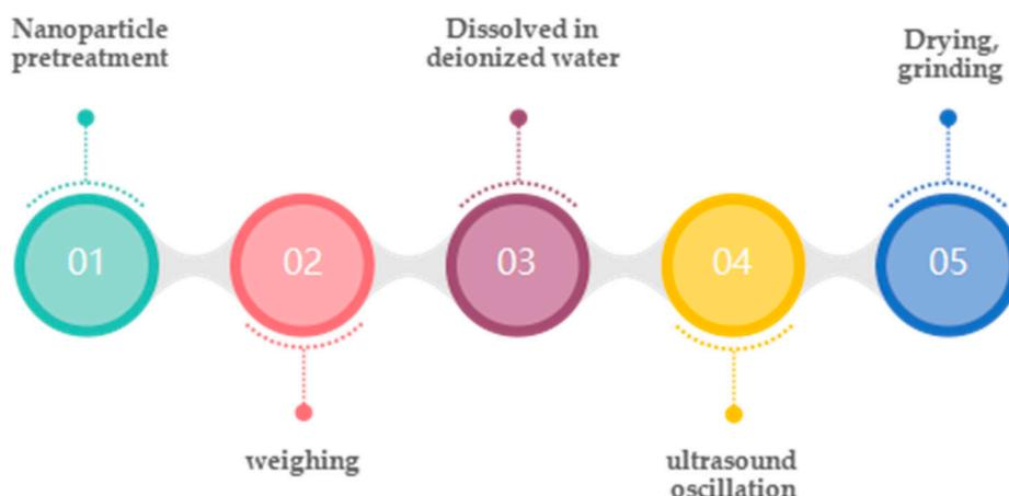
**Figure 3.** Two-step preparation of molten salt nanofluidic flow [57].
