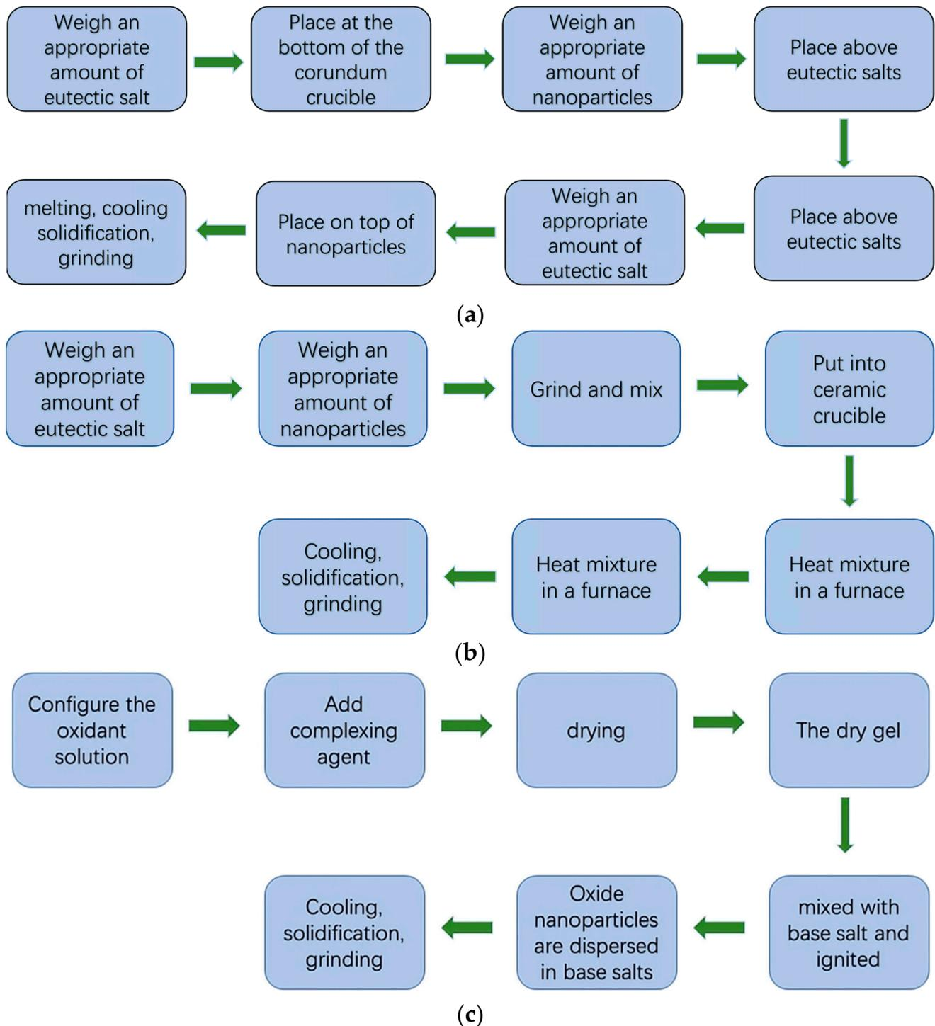
**Figure 2.** One-step preparation of molten salt nanofluidic flow. (a) Dissolution method; (b) In situ synthesized; (c) Sol-gel self-combustion method.
