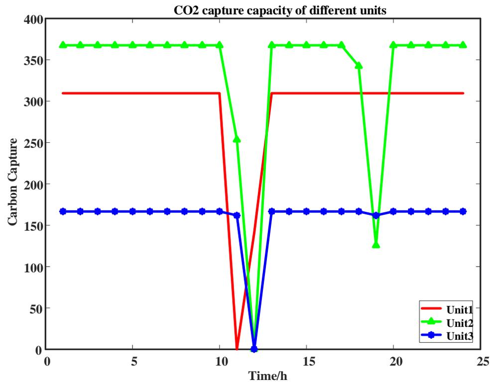
Figure 5. CO<sub>2</sub> capture capacity of different units.
