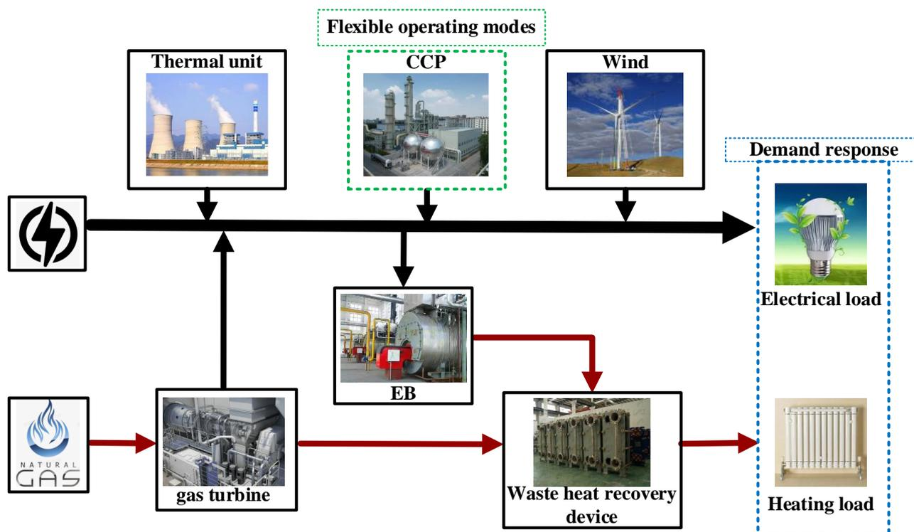
Figure 1. Structure diagram of IEHS.
