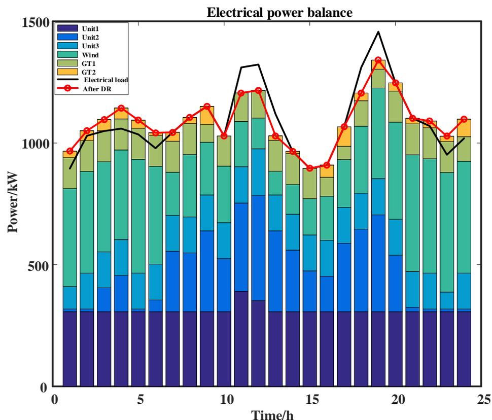
Figure 9. Electrical power balance.
