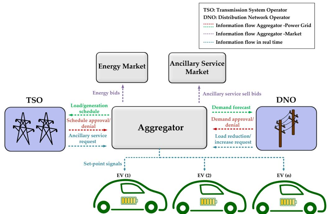
Figure 8. Centralized control architecture of EV charging [15].
