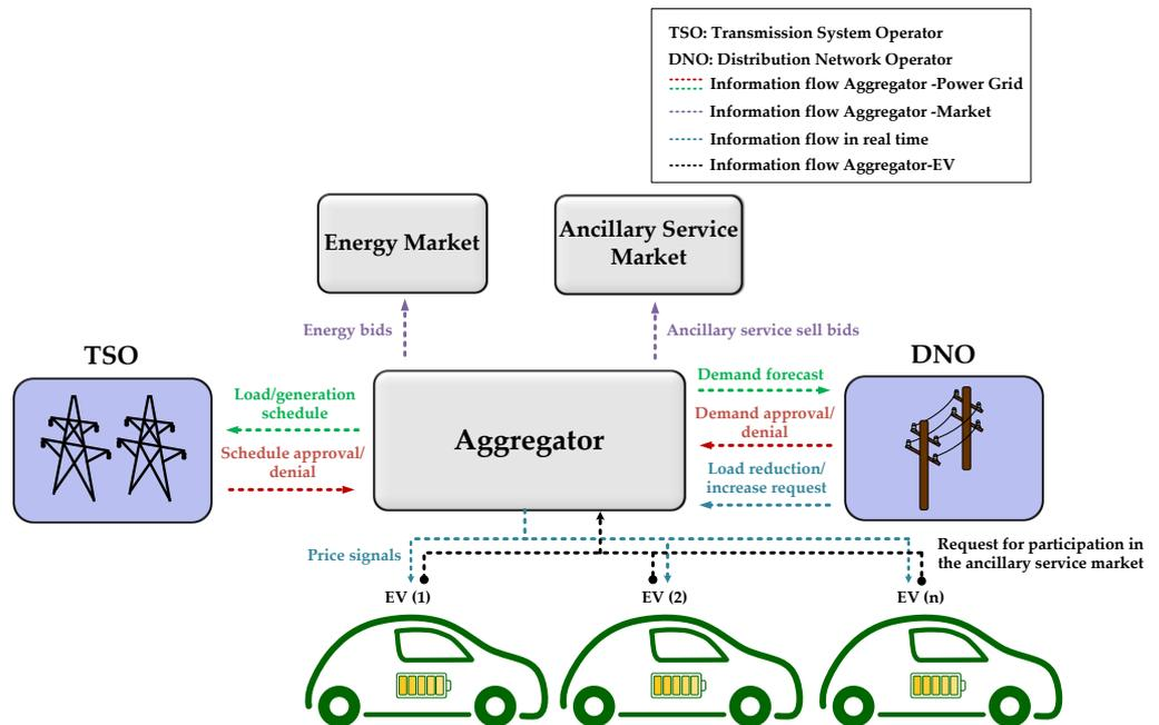
Figure 9. Decentralized control architecture of EV charging [15].
