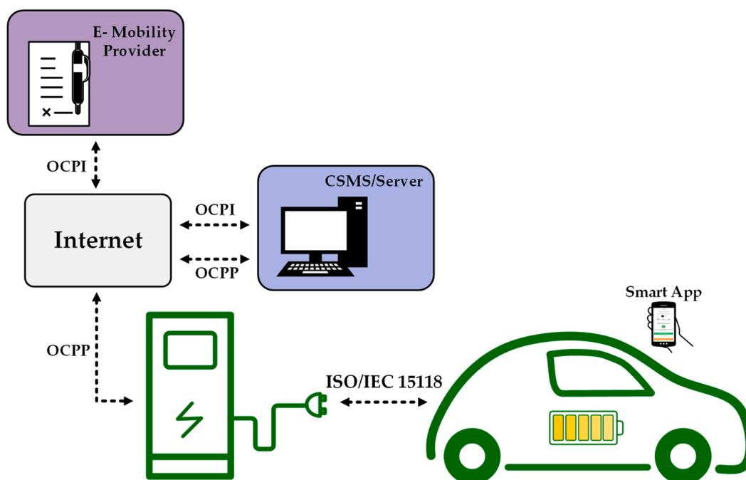
**Figure 11.** Communication protocols used during the charging procedure.
