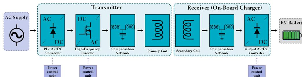
**Figure 4.** Block diagram of a unidirectional inductive charger.
