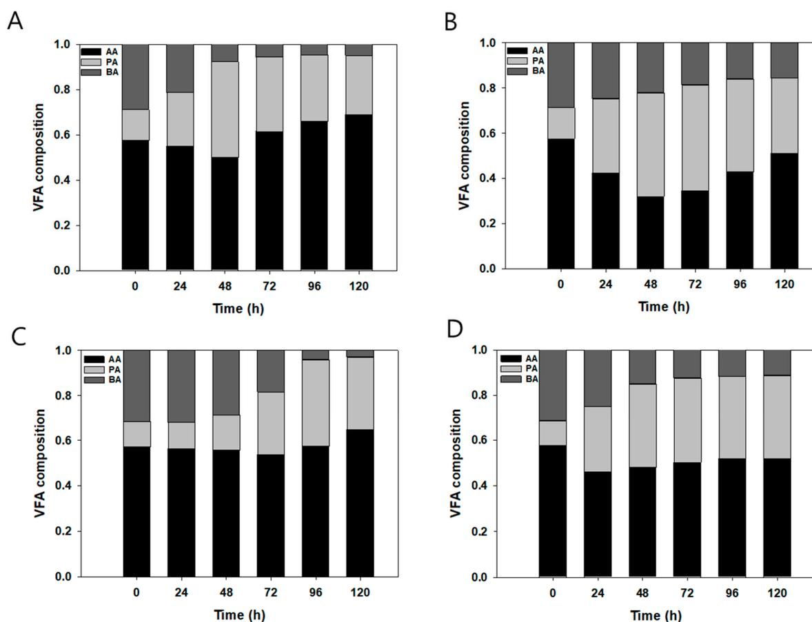
**Figure 5.** VFA composition under each condition (initial VFA composition was 60% AA, 10% PA, and 30% BA): (A) 2 g/L and pH 5.5, (B) 2 g/L and pH 7.0, (C) 5 g/L and pH 5.5, and (D) 5 g/L and pH 7.0. VFA solutions were fed manually after 63 h in order to maintain the concentration at 2 g/L and pH 5.5.
