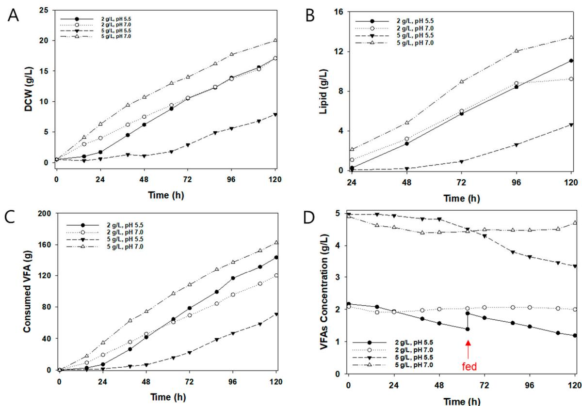
**Figure 4.** Effects of initial VFA concentration and pH on the growth of *C. curvatus* using the automatic fed-batch mode cultivation: (A) dry cell weight, (B) lipid, (C) consumed VFA, and (D) VFA concentration in broth. The red arrow indicates when a VFA was added.
