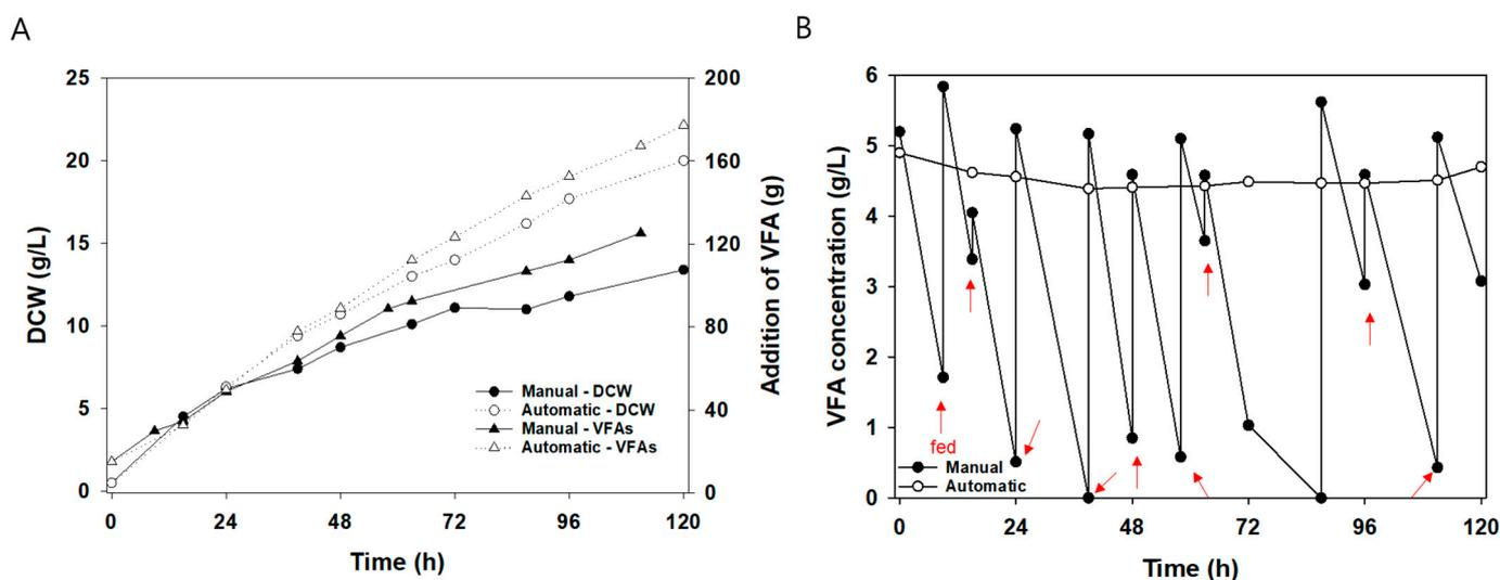
**Figure 3.** Two fed-batch cultivation modes with *C. curvatus*: (A) Dry cell weight and addition of VFA amount; (B) VFA concentration in broth. pH-stat for manual feeding used 5 N HCl as an acidic agent, and VFA solution was added ten times for fed-batch. The red arrows indicate when a VFA was added. Automatic feeding used 500 g/L VFA solution to obtain a pH of 7.0. The initial VFA concentration was 5 g/L.
