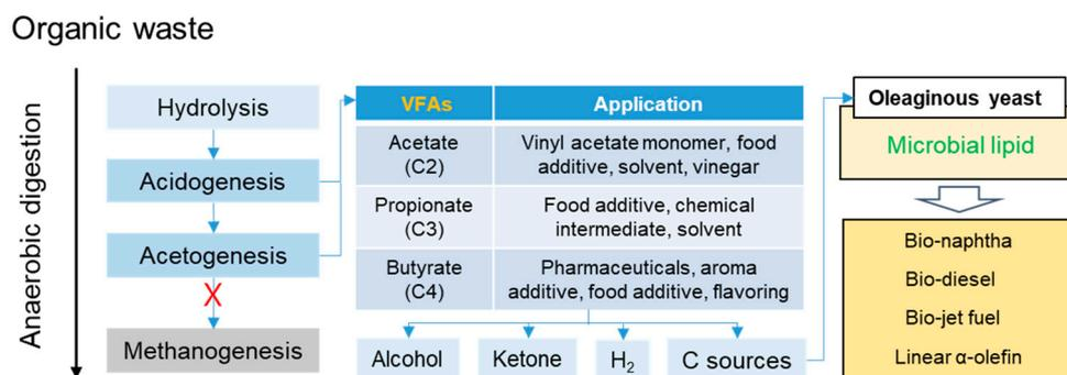
**Figure 1.** Product technology of VFAs and microbial lipid platforms.
