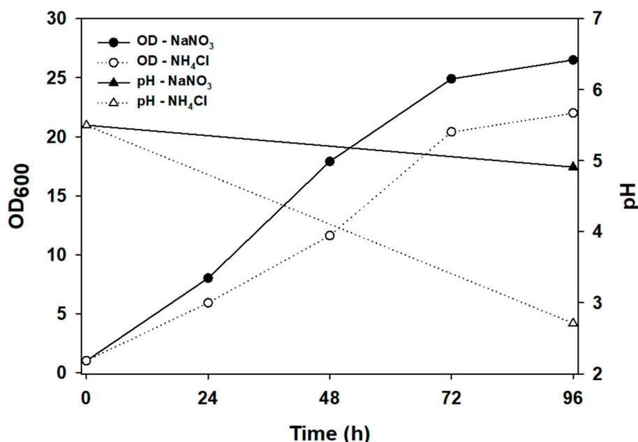
**Figure 2.** Effects of cell growth and pH change on the different nitrogen sources. Glucose (30 g/L) was used as the sole carbon source at a C/N of 40 in flask culture. Initial pH and rotation speed were 5.5 and 180 rpm, respectively.
