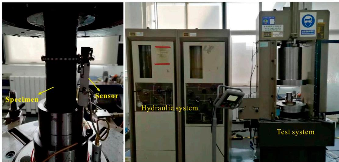
Figure 2. MTS815 test system.
