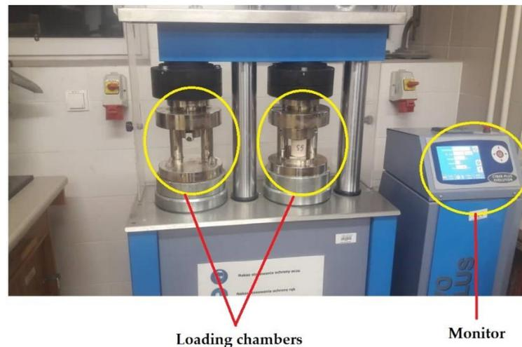
**Figure 3.** The UCS measurement apparatus.
