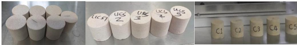
**Figure 2.** Appearance of the sandstone samples for the UCS test: dry samples (right), wet samples (middle), for the AVS test (left).
