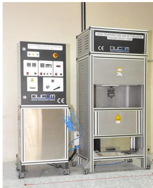
Figure 2. Photograph of air-jet erosion tester facility.
