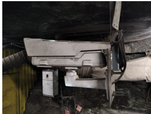
Figure 2. Measuring equipment—RGB camera to monitor the working conditions of the transfer point.
