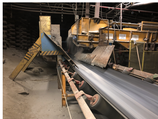
Figure 1. Research object—perpendicular, angular transfer point in an underground copper ore mine.
