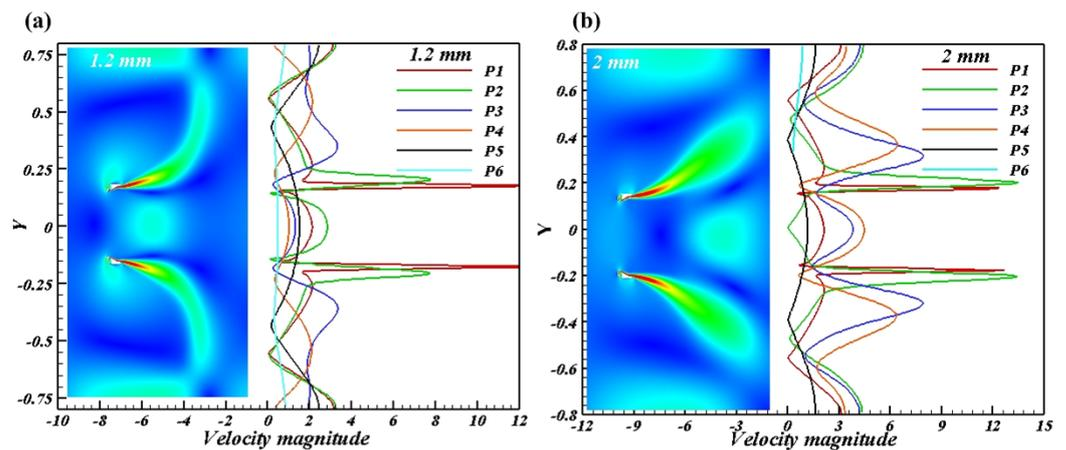
Figure 8. Velocity Profile and contours (a) 1.2 mm slit thickness at 3 m/s inlet velocity. (b) 2 mm slit thickness at 6 m/s inlet velocity.
