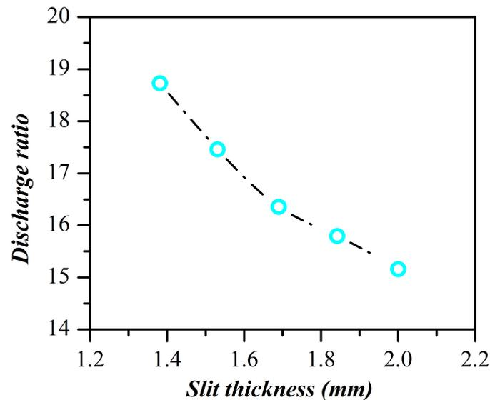
**Figure 17.** Slit thickness vs. Discharge ratio.
