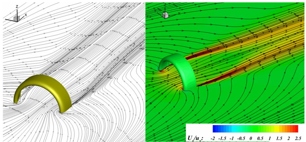
Figure 12. Streamline and Velocity contours of 1.2 mm slit thickness ( $V = 3$  m/s).
