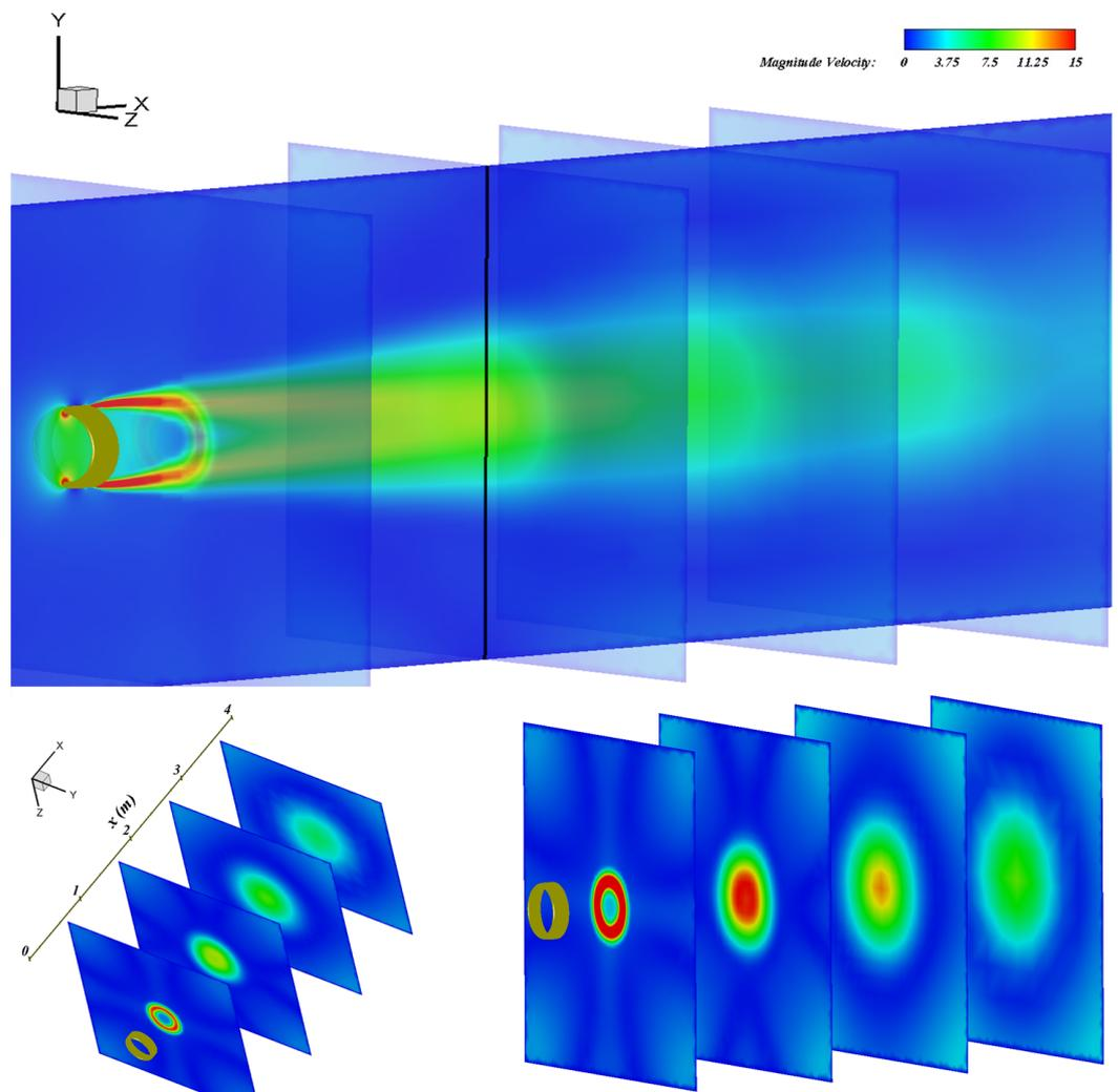
Figure 13. Perspective view of airflow at downstream of 1.2 mm slit thickness with 3 m/s inlet velocity.
