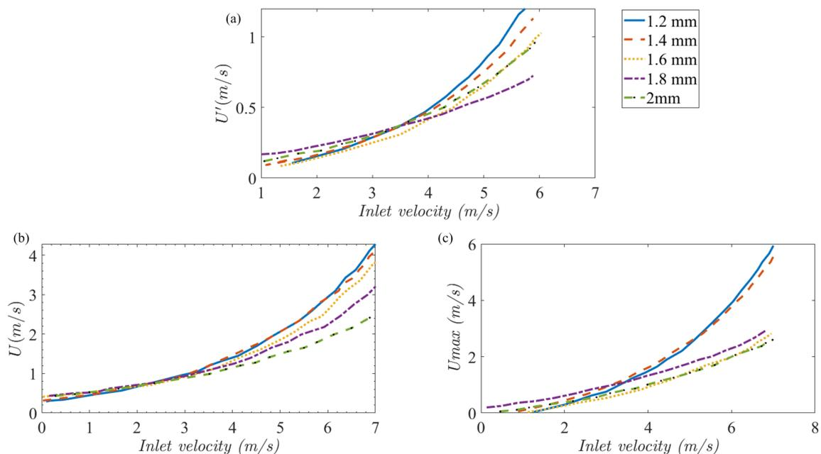
**Figure 10.** (a) Average velocity ( $\bar{U}$ ) at a distance of 0.9 m from the outlet slit (b) Standard deviation of velocity ( $U'$ ) at a distance of 0.9 m from the outlet slit (c) Maximum velocity ( $U_{max}$ ) at a distance of 0.9 m from the outlet slit.
