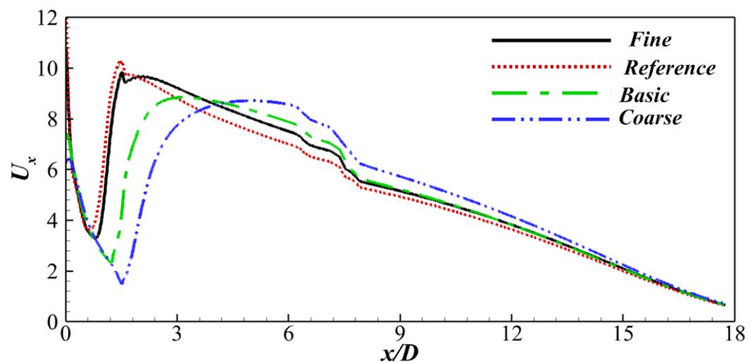
Figure 3. Velocity profile at the downstream of the fan with different  $y^+$  values .
