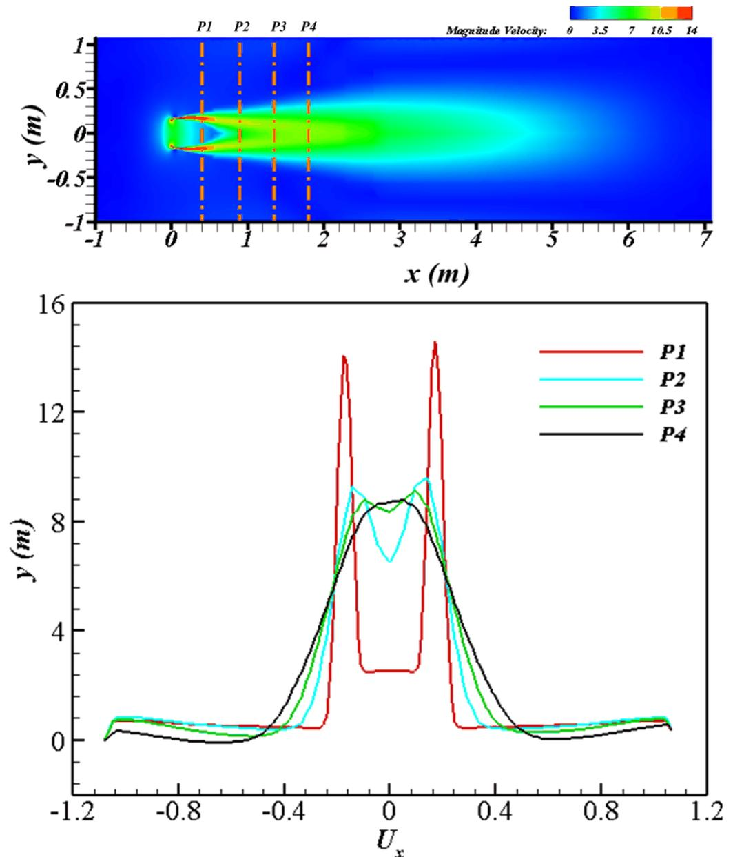
**Figure 14.** Perspective view of airflow downstream of 1.2 mm slit thickness with 3 m/s inlet velocity.
