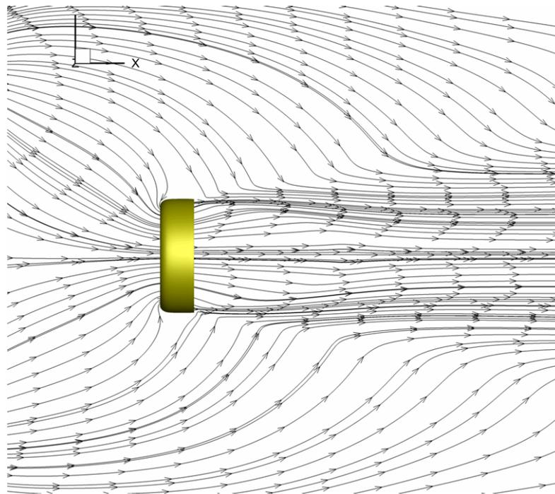
**Figure 15.** Velocity Vectors displaying the direction of output air in the 3D domain at a distance of 0.9 m from the fan.
