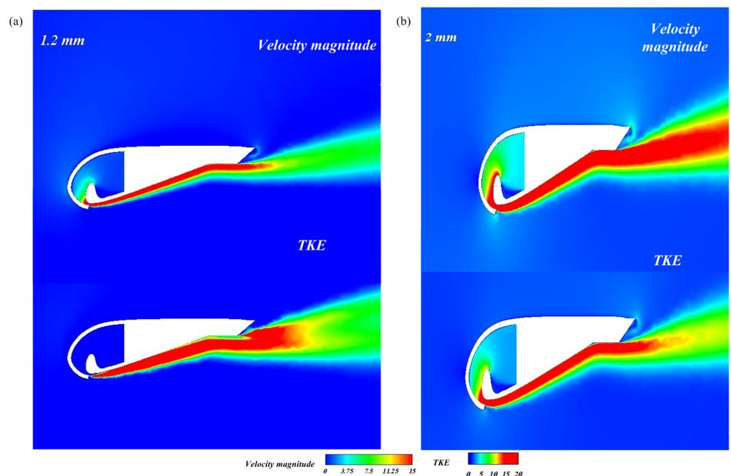
**Figure 11.** Velocity magnitude (m/s) and Turbulent Kinetic Energy ( $\text{m}^2 \cdot \text{s}^{-2}$ ) from the slit (a) 1.2 mm (b) 2 mm thickness.
