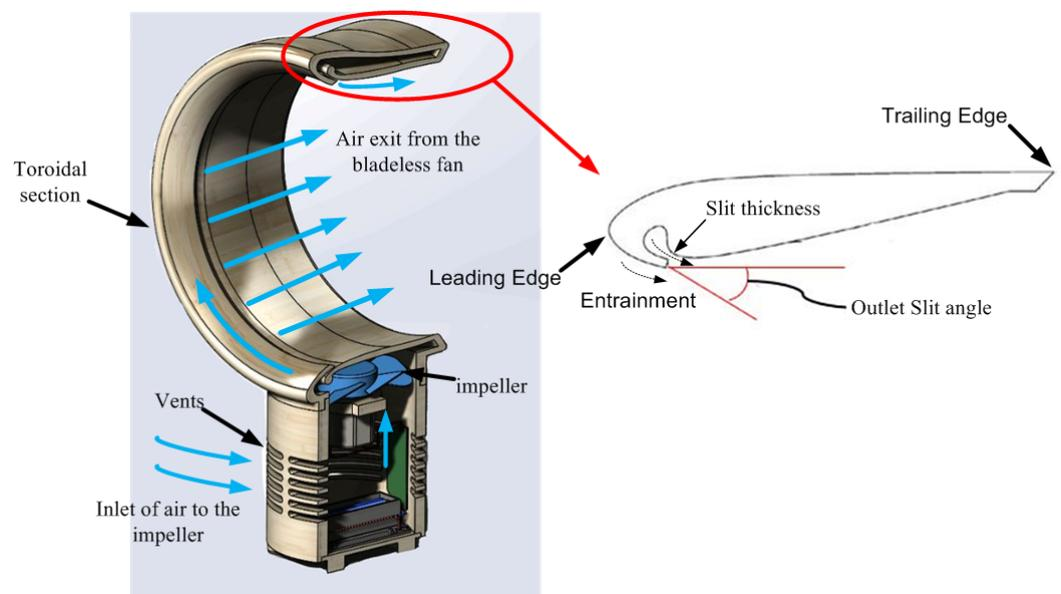
**Figure 1.** Eppler 473 Airfoil Profile with the depiction of outlet slit and height of cross-section.
