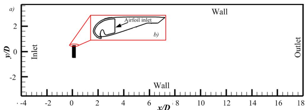
**Figure 2.** (a) Fluid Domain Boundary Conditions. (b) Airfoil Boundary condition.
