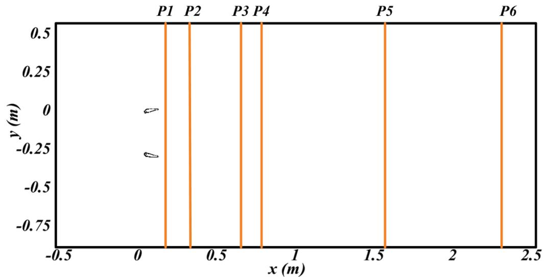
Figure 7. Reference lines in the 2D domain for measuring properties of fluid flow.
