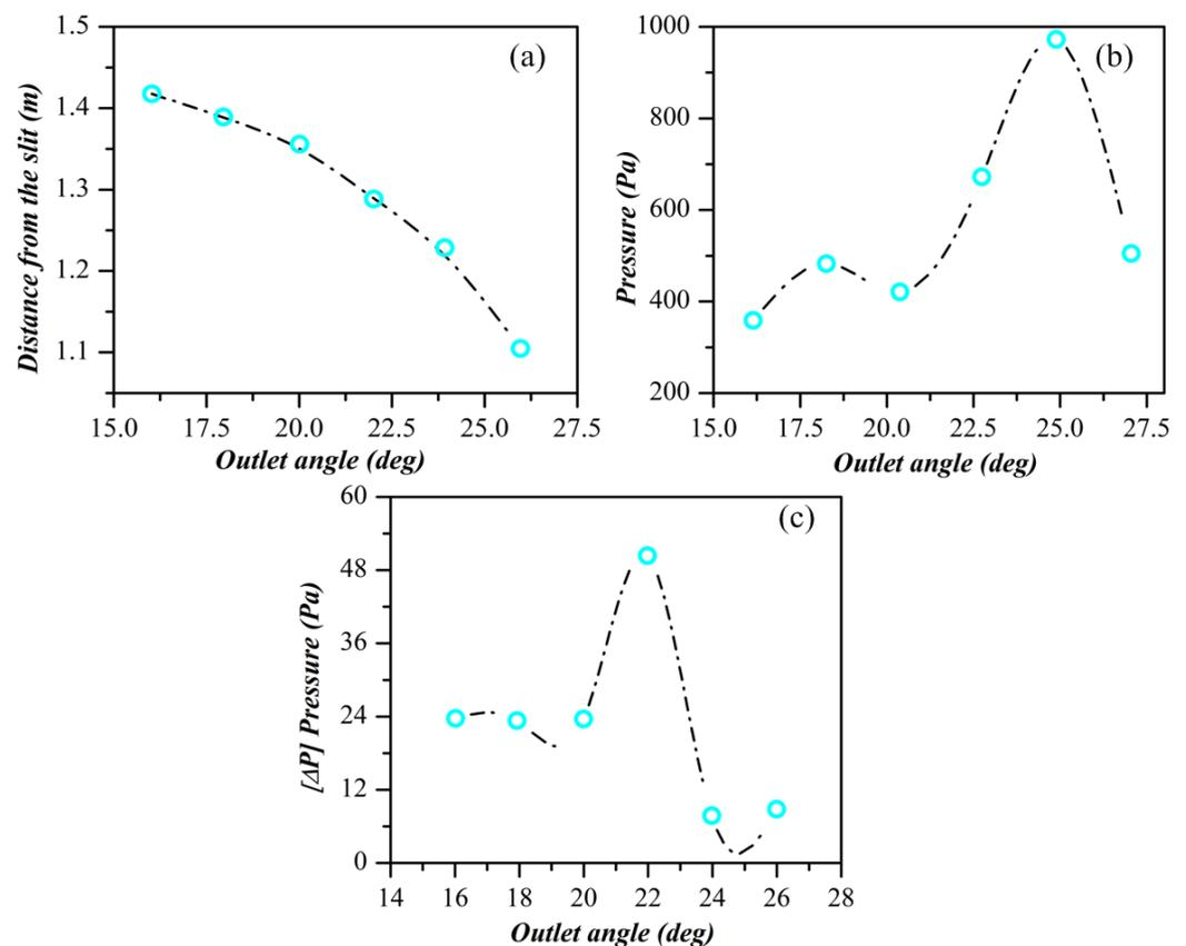
**Figure 18.** (a) Converging distance for different outlet angles, (b) Pressure difference between the slit and leading edge for different outlet angles and (c) Pressure difference between the trailing and leading edge for different outlet angle.
