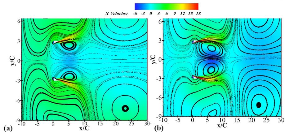
**Figure 9.** Streamline flow distribution 2D (a) 1.2 mm slit thickness at 3 m/s inlet velocity. (b) 2 mm slit thickness at 6 m/s inlet velocity.
