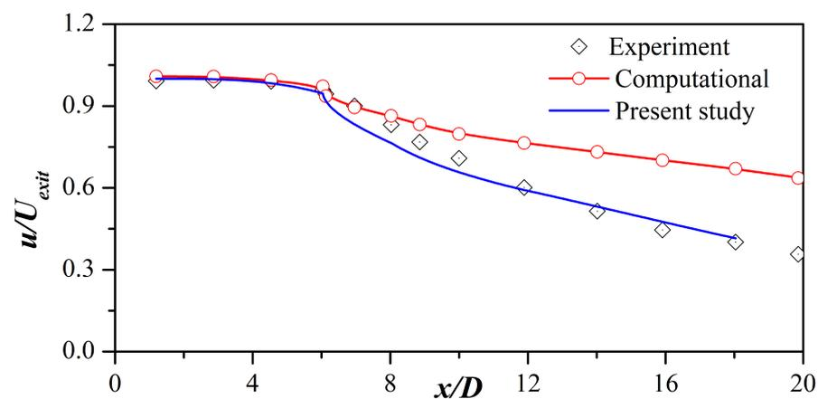
**Figure 6.** Comparison of downstream velocity validated with Computational by Jafari et al. [4], and experiment by Quinn [5].
