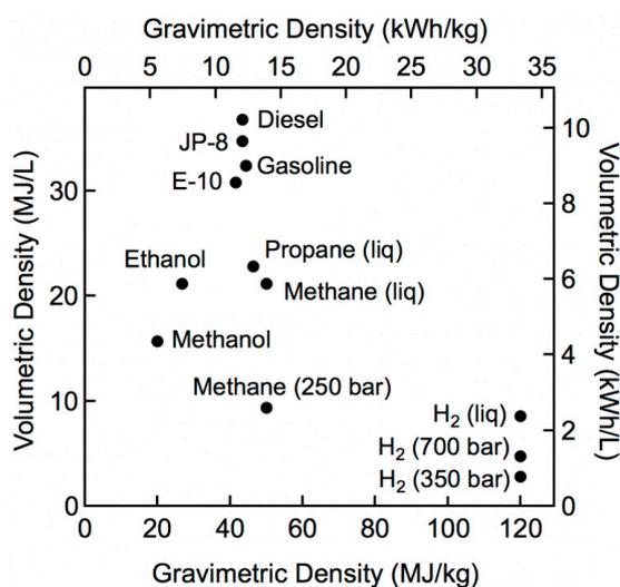
**Figure 1.** Comparison of specific energy (energy per mass or gravimetric density) and energy density (energy per volume or volumetric density) for several fuels based on lower heating values. After [14].
