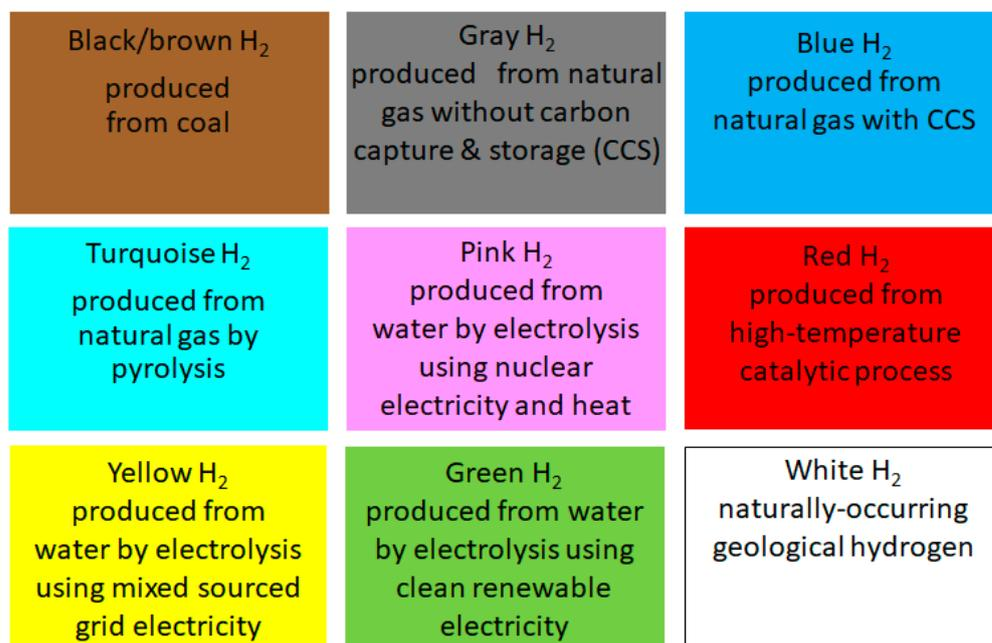
**Figure 3.** The spectrum of H<sub>2</sub> production processes.
