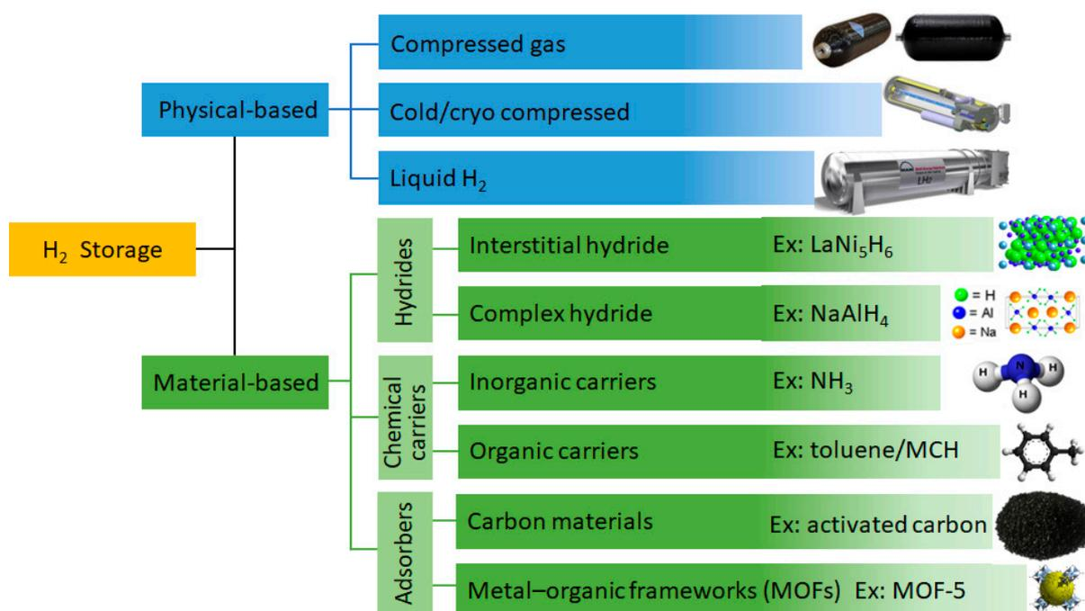
**Figure 5.** Overview of H<sub>2</sub> storage technologies.
