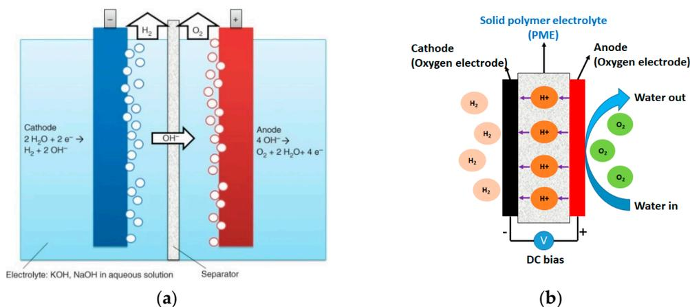
**Figure 4.** (a) H<sub>2</sub> generation from alkaline electrolyzer. Reproduced with permission from [58], John Wiley and Sons, 2022; and (b) schematics of PEM water electrolyzer (Solid polymer electrolyte membrane is the same as proton exchange membrane).
