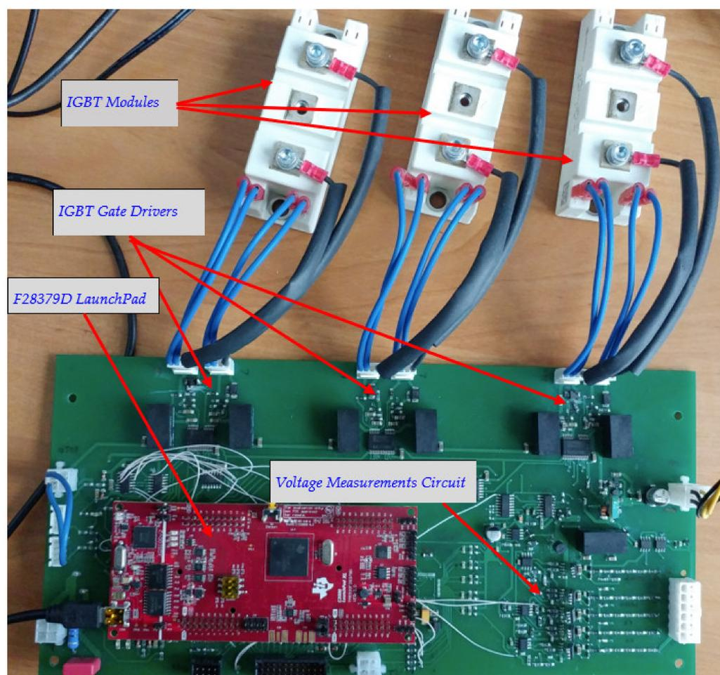
**Figure 4.** View of the APF control circuit during the development process (during desktop testing).
