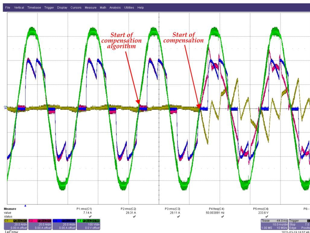
**Figure 16.** Experimental waveforms of the APF in transition state, line current  $i_{M1}(t)$  (red), load current  $i_{L1}(t)$  (blue), compensation current  $i_{C1}(t)$  (yellow), and line voltage  $u_{M1}(t)$  (green).
