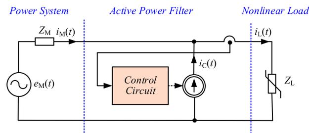
**Figure 1.** Block diagram of APF.
