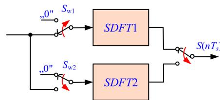
Figure 8. Block diagram of stable “switching” SSDFT.
