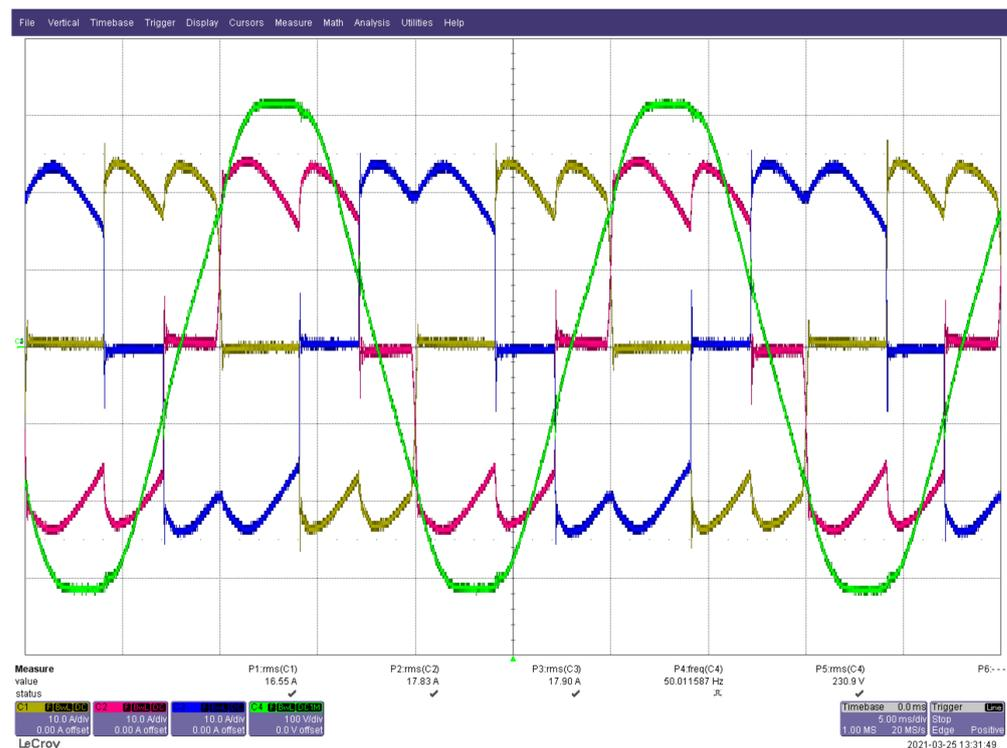
**Figure 14.** Exemplary experimental waveforms for fully controlled rectifier, load currents  $i_{L1}(t)$  (red),  $i_{L2}(t)$  (blue),  $i_{L3}(t)$  (yellow), and line voltage  $u_{M1}(t)$  (green).
