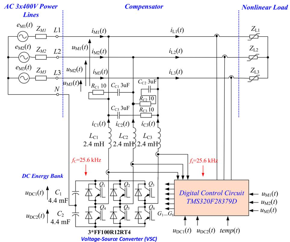
Figure 2. Three-phase active power filter compensation circuit.
