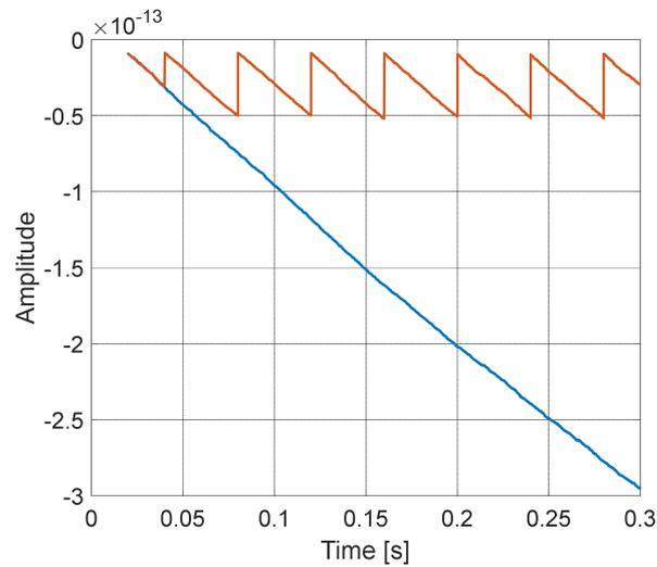
Figure 9. Error amplitudes on the output of first harmonic detector. Classical (blue curve), switching (red curve).
