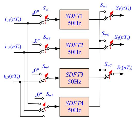
Figure 10. Block diagram of three-phase first harmonic detectors using stable SSDFT.
