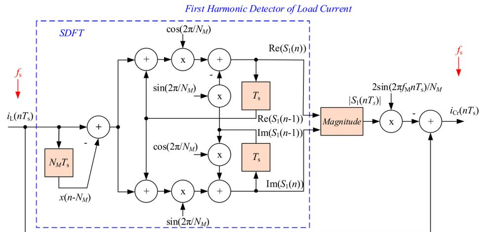
Figure 7. Block diagram of circuit for calculating compensation current.
