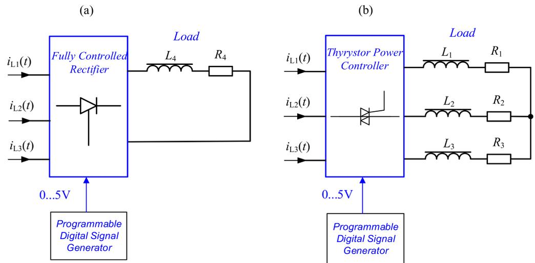
**Figure 12.** Three-phase nonlinear loads: (a) with fully controlled rectifier, (b) with thyristor power controller.
