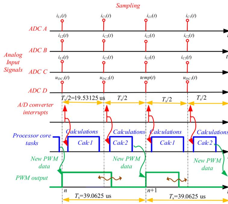
**Figure 6.** Timing diagram of data flow in the APF controls circuit.
