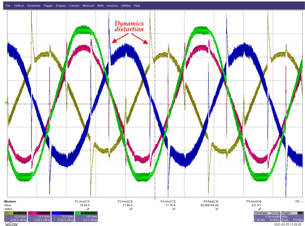
**Figure 15.** Exemplary experimental waveforms for fully controlled rectifier, APF is switch on, line currents:  $i_{M1}(t)$  (red),  $i_{M2}(t)$  (blue),  $i_{M3}(t)$  (yellow), and line voltage  $u_{M1}(t)$  (green).
