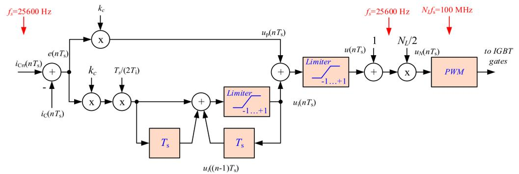
Figure 5. Simplified block diagram of digital PI current controller.
