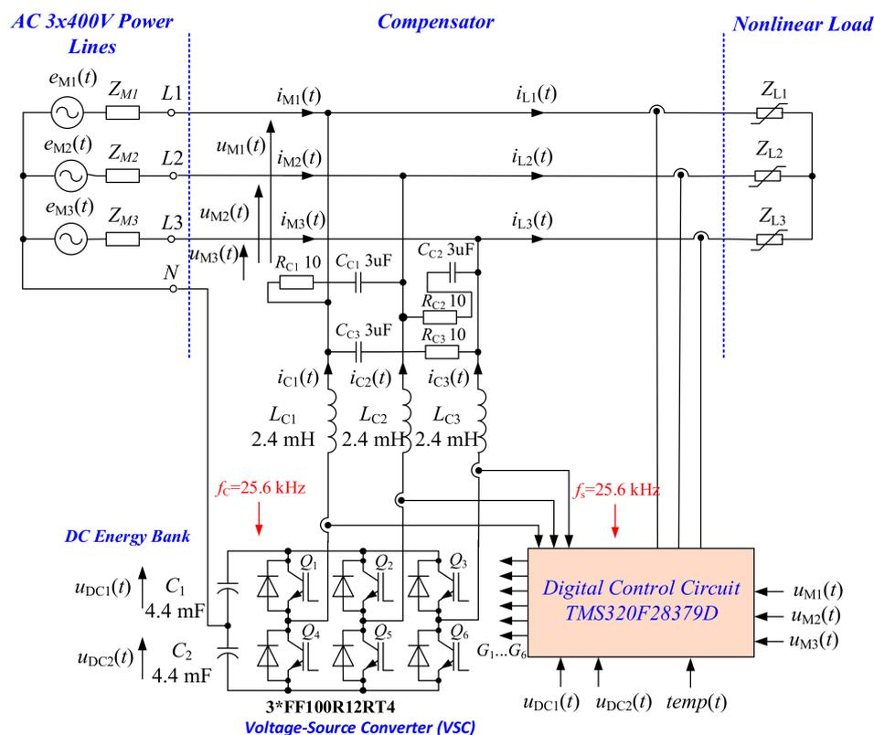
Figure 2. Three-phase active power filter compensation circuit.
