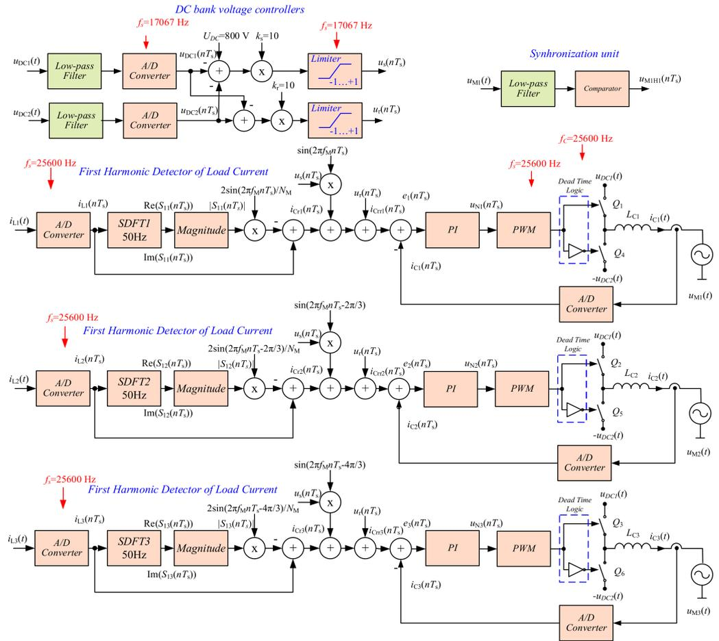
Figure 3. Simplified block diagram of APF control algorithm.
