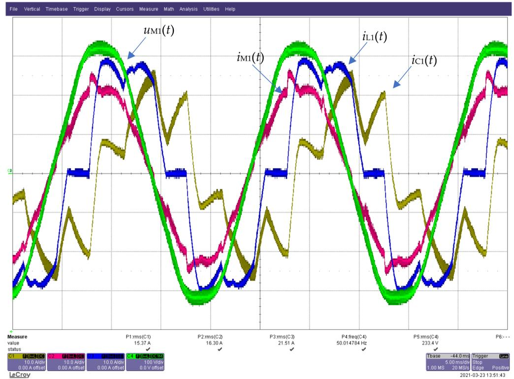
**Figure 13.** Exemplary experimental waveforms of the APF in steady state: line current  $i_{M1}(t)$ , compensation current  $i_{C1}(t)$ , load current  $i_{L1}(t)$ , and line voltage  $u_{M1}(t)$ .
