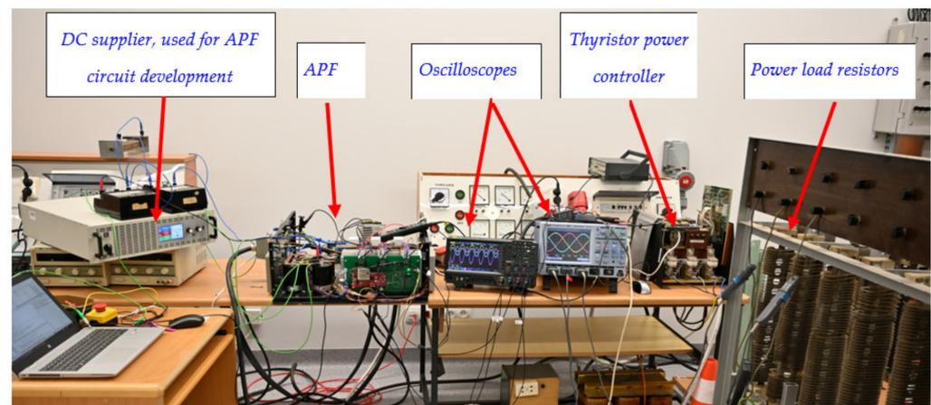
Figure 11. A view of the APF laboratory setup.
