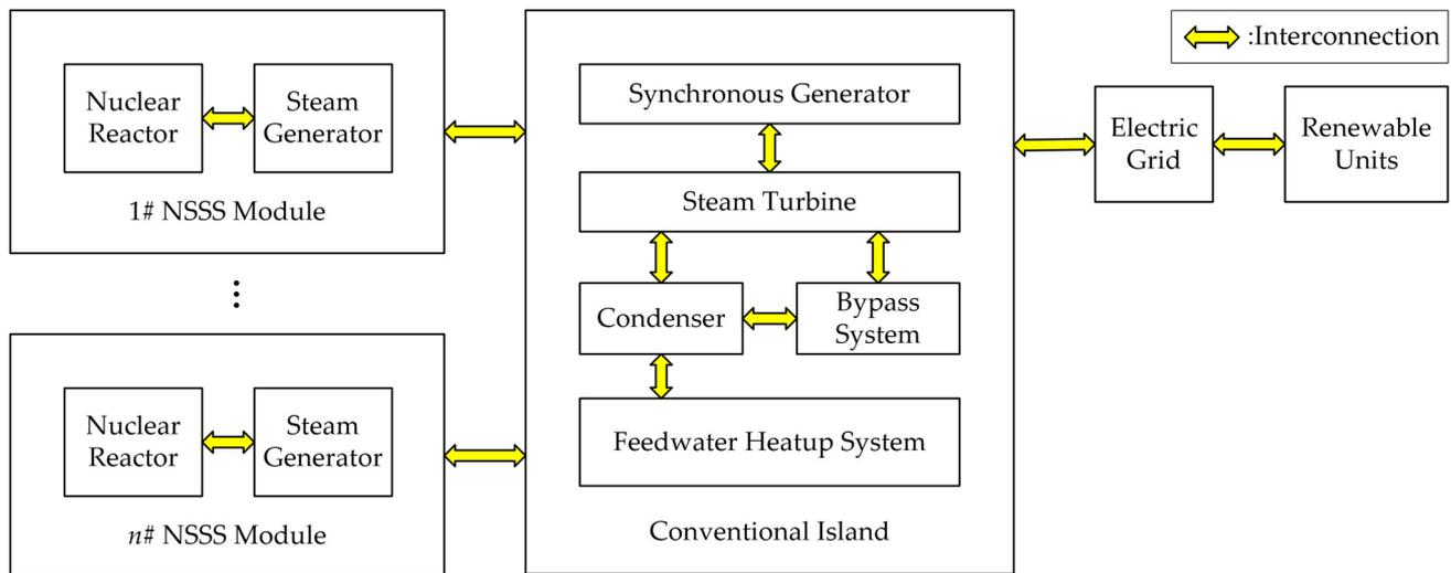
**Figure 5.** Interconnection amongst systems and equipment of a multimodular mHTGR plant.
