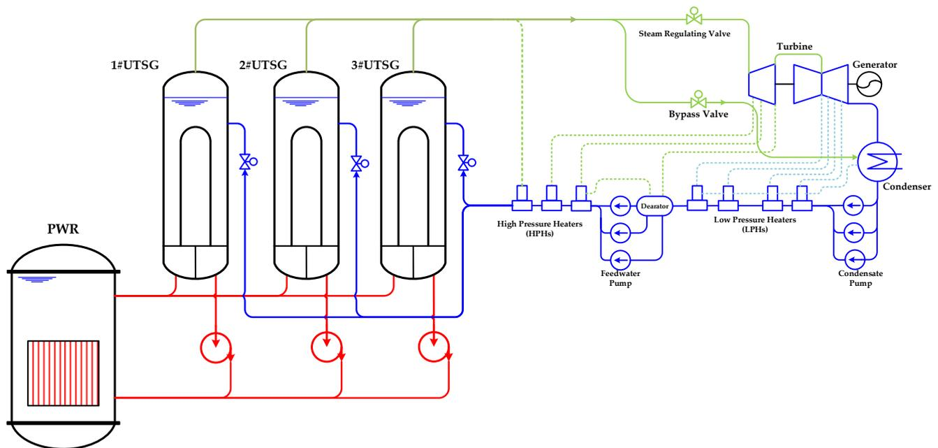
**Figure 1.** Schematic diagram of a single-modular PWR plant, UTSG: U-tube steam generator. The red lines denote the primary coolant, the blue lines denote the secondary coolant in liquid state, and the green lines denotes the secondary coolant in steam state.
