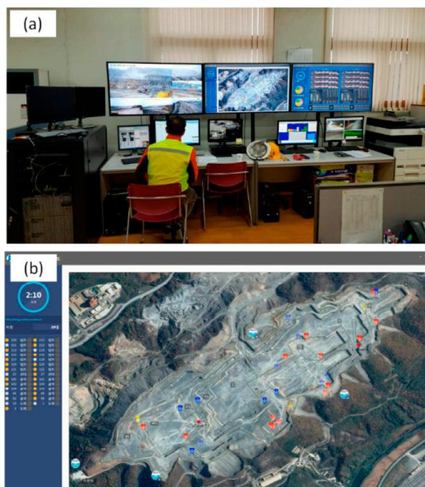
**Figure 10.** An open-pit mine in South Korea with a wireless communications system for fleet management of mine equipment. (a) Control center. (b) Main dashboard (Reprinted from Ref. [65]).
