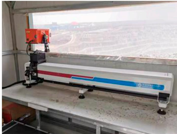
**Figure 9.** The Frequency Modulated Continuous Wave Ground-Based Synthetic Aperture Radar (FMCW-GBSAR) System from NCUT (Reprinted from Ref. [63]).
